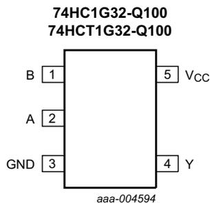
Fig 4. Pin configuration
