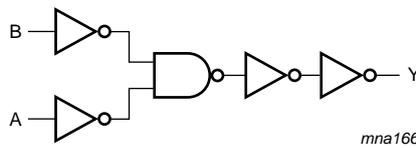
Fig 3. Logic diagram
