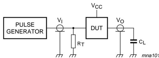
Measurement points are given in [Table 8](#). Definitions for test circuit:
