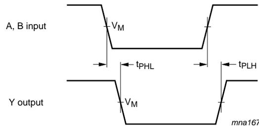
For 74HC1G32-Q100:  $V_M = 0.5 \times V_{CC}$ ;  $V_I = GND\text{ to }V_{CC}$
