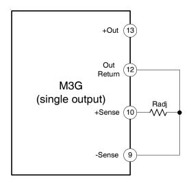
Fig 4. Configuration for Adjusting Single Output Voltage from 0 to +0.25V
