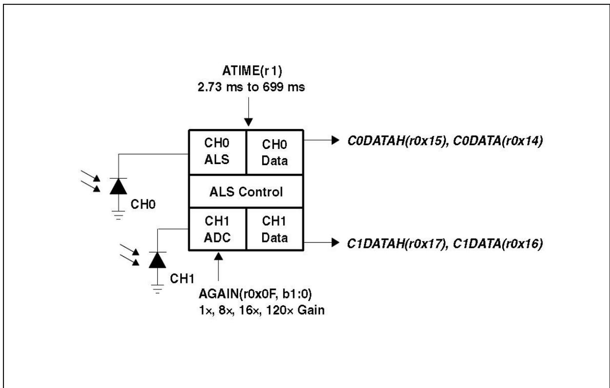
The registers for programming the integration and wait times are a 2's complement values. The actual time can be calculated as follows:
