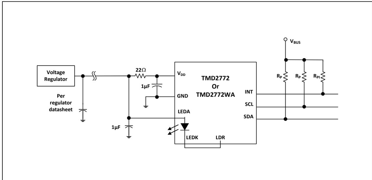
$V_{BUS}$  in the above figures refers to the I<sup>2</sup>C bus voltage which is either  $V_{DD}$  or 1.8V. Be sure to apply the specified I<sup>2</sup>C bus voltage shown in the Available Options table for the specific device being used.
