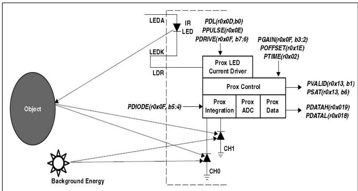
The LED current driver, output on the LDR terminal, provides a regulated current sink that eliminates the need for an external current limiting resistor. The combination of proximity LED drive strength (PDRIVE) and proximity drive level (PDL) determine the drive current. PDRIVE sets the drive current to 100%, 50%, 25%, or 12.5% when PDL is not asserted. However, when PDL is asserted, the drive current is reduced by a factor of 9.
