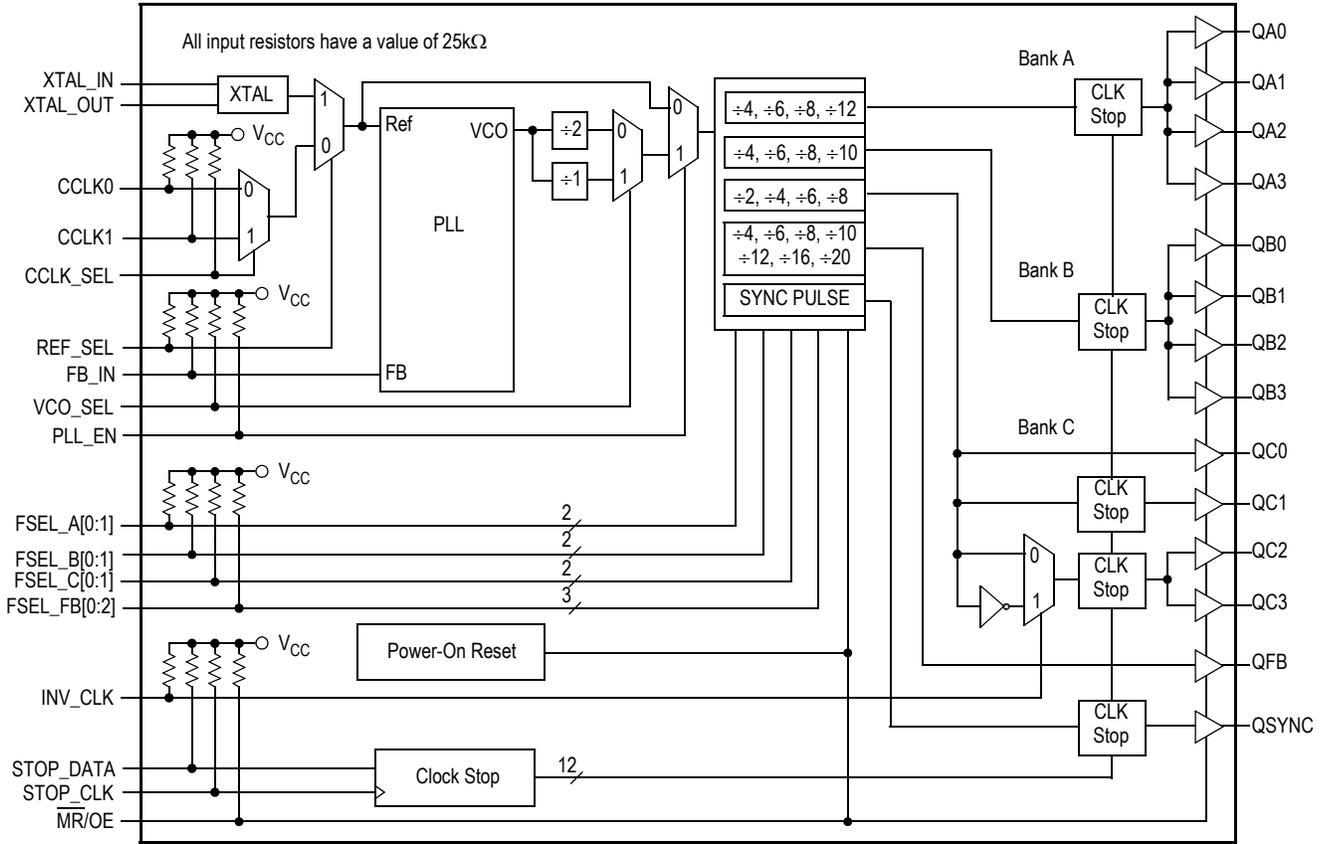
Figure 1. Logic Diagram
