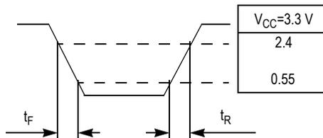
**Figure 22. Output Transition Time Test Reference**
