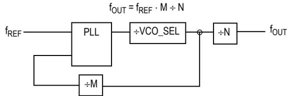
where  $f_{REF}$  is the reference frequency of the selected input clock source (CCLK0, CCLK1 or XTAL interface),  $M$  is the PLL feedback divider and  $N$  is a output divider. The PLL feedback divider is configured by the FSEL\_FB[2:0] and the output dividers are individually configured for each output bank by the FSEL\_A[1:0], FSEL\_B[1:0] and FSEL\_C[1:0] inputs.
