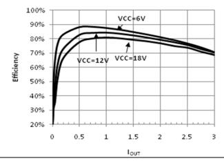
Figure 2.10 Efficiency vs. Output Current (VOUT = 3.3V)
