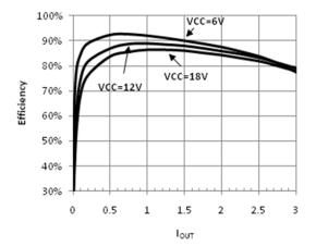
Figure 2.11 Efficiency vs. Output Current ( VOUT = 5V)
