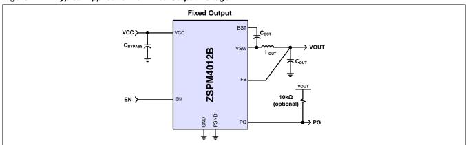
High Efficiency 2A Synchronous Buck Converter
