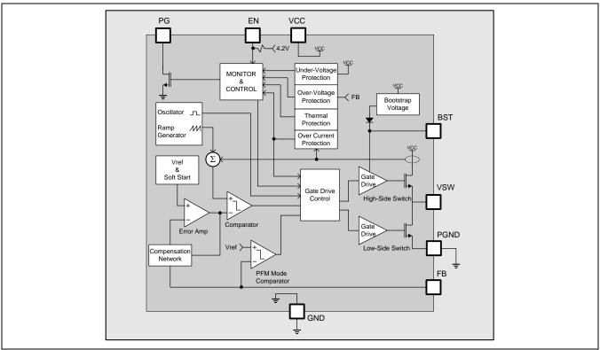
High Efficiency 2A Synchronous Buck Converter
