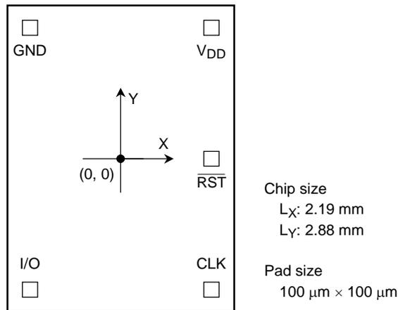
**Pad Coordinates** (μm, μm)
