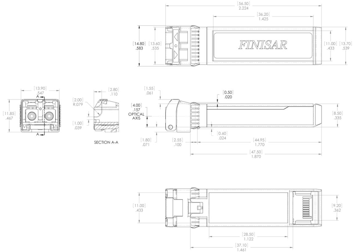
**Figure 2. FTLX8573D3BTL Mechanical Dimensions.**
