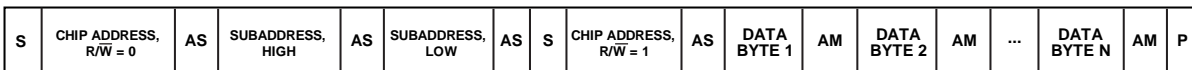
S = START BIT, P = STOP BIT, AM = ACKNOWLEDGE BY MASTER, AS = ACKNOWLEDGE BY SLAVE. SHOWS A ONE-WORD WRITE, WHERE EACH WORD HAS N BYTES.
