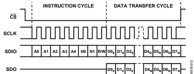
Figure 39. Serial Register Interface Timing, LSB First
