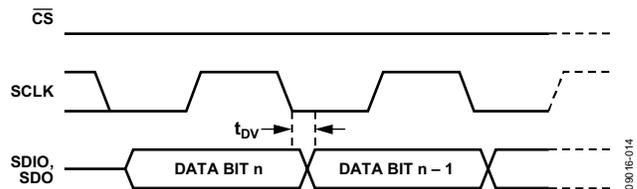
Figure 41. Timing Diagram for Serial Port Register Read
