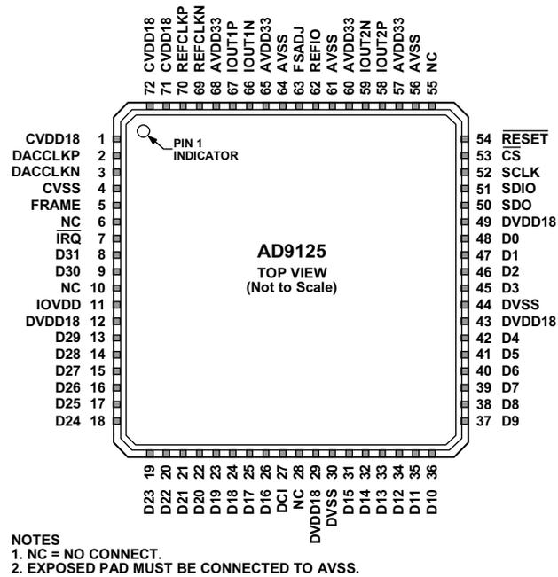
Figure 3. Pin Configuration
