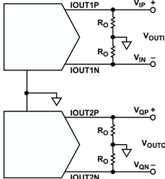
Figure 68. Basic Transmit DAC Output Circuit
