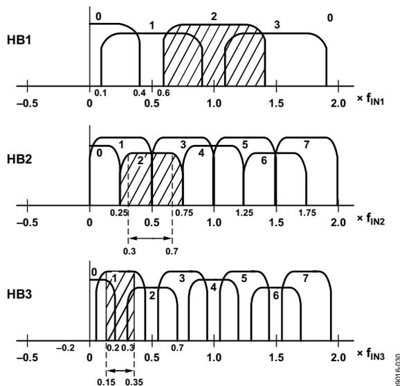
Figure 60. Signal Propagation for 8× Interpolation ( $f_{DATA}$  Modulation)
