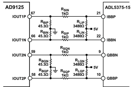
Figure 74. Passive Level-Shifting Network for Biasing ADL5375-15
