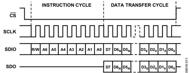
Figure 38. Serial Register Interface Timing, MSB First
