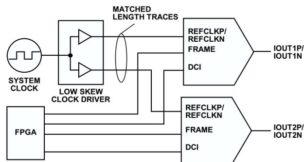
Figure 81. Typical Circuit Diagram for Synchronizing Devices
