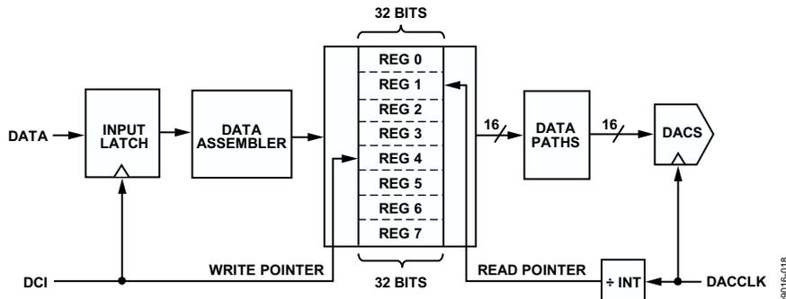
Figure 47. Block Diagram of Datapath Through FIFO
