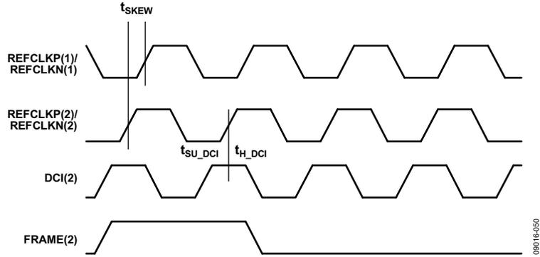
Figure 82. Timing Diagram Required for Synchronizing Devices
