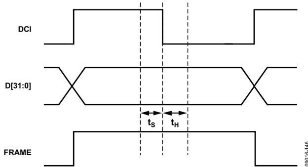
Figure 45. Timing Diagram for Input Data Ports
