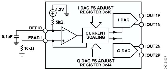
Figure 66. Simplified Block Diagram of DAC Core
