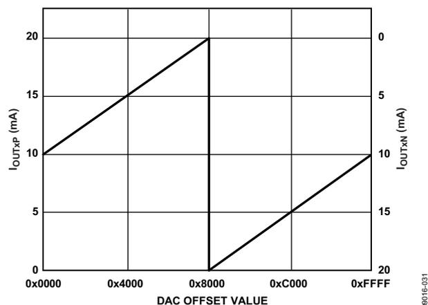
Figure 61. DAC Output Currents vs. DAC Offset Value
