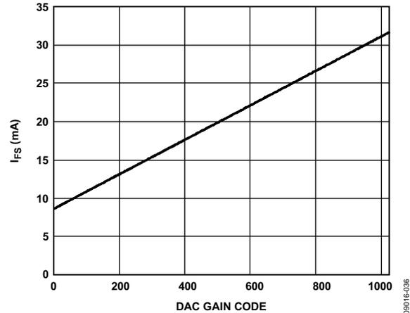
Figure 67. DAC Full-Scale Current vs. DAC Gain Code
