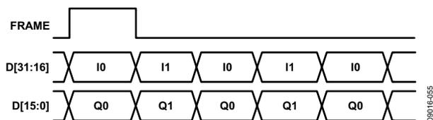
Figure 87. Timing Diagram for Dual-Word Mode SED Operation
