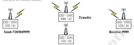
• If you want to send data 9999 from equipment which UID=01 through equipment which UID=03 to transfer to equipment which UID=04 and transfer again to equipment which UID=02, data format which you send is 0x730304029999.
