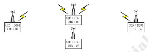
Or, command is 0xC00204 when  $UID=01 \rightarrow UID=02 \rightarrow UID=04$ .
