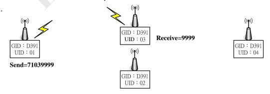
If you want to send data 9999 from equipment which UID=01 through equipment which UID=03 to transfer to equipment which UID=04, data format which you send is 0x7203049999.
