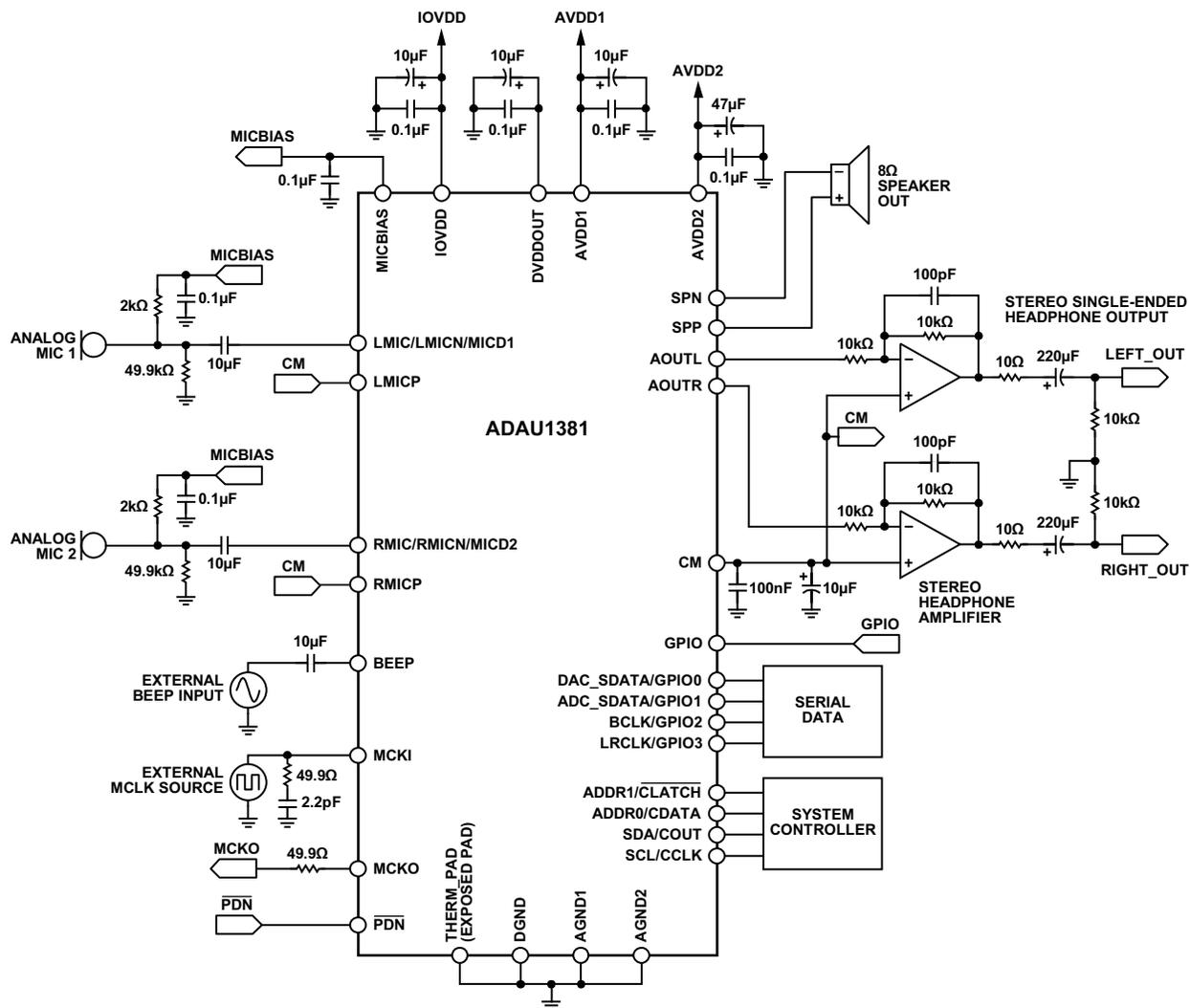
Figure 24. System Block Diagram with Analog Microphone Inputs
