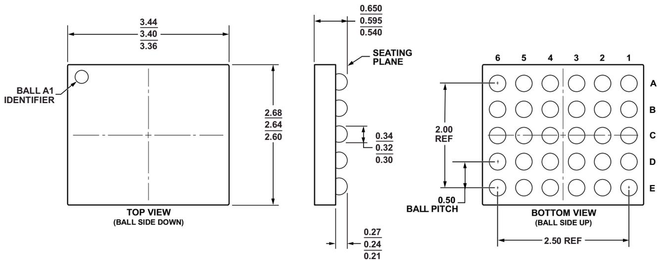
Figure 74. 30-Ball Wafer Level Chip Scale Package [WLCSF]
