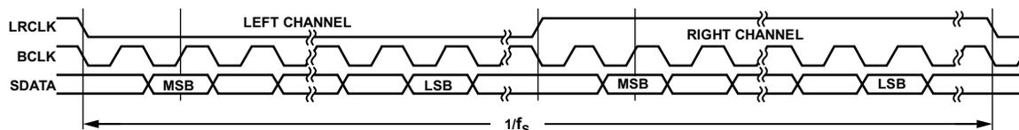
Figure 47. I²S Mode—16 Bits to 24 Bits per Channel
