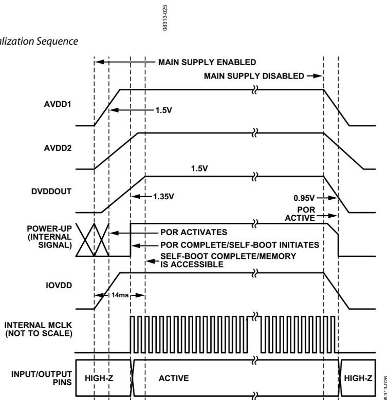
Figure 28. Power-Up and Power-Down Sequence Timing Diagram
