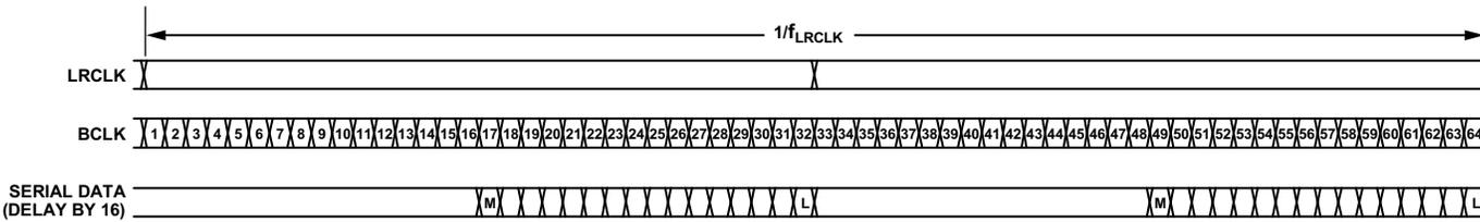
Figure 67. Serial Audio Data Delay by 16 Example
