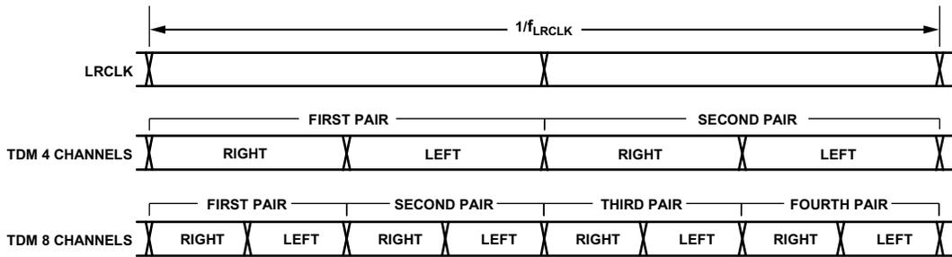
Figure 64. Right First Channel Selection in TDM
