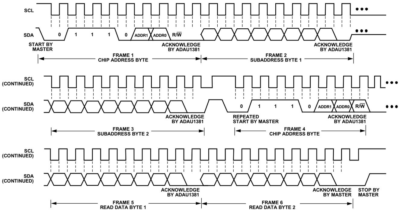
Figure 39. I<sup>2</sup>C Read from ADAU1381 Clcking
