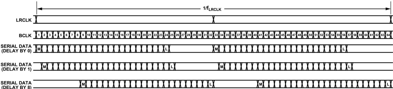
Figure 66. Serial Audio Data Delay Example Settings
