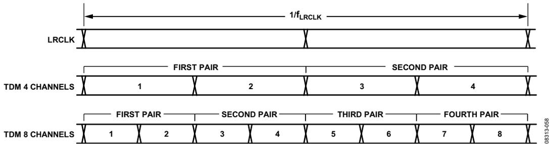
Figure 60. TDM Channel Pairs
