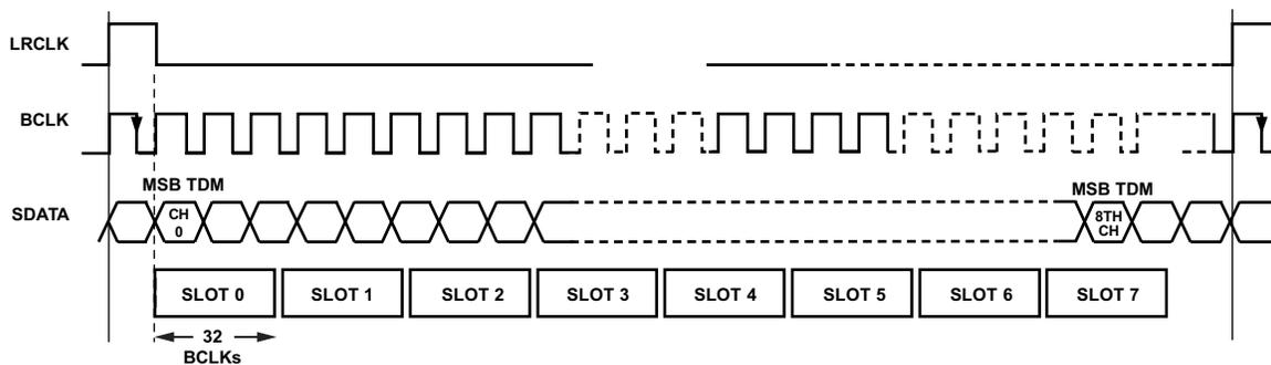
Figure 51. TDM Mode with Pulse Word Clock
