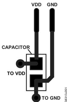
Figure 53. Recommended Power Supply Bypass Capacitor Layout
