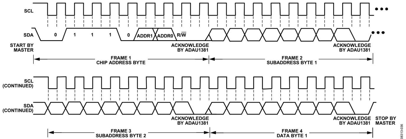
Figure 38. I<sup>2</sup>C Write to ADAU1381 Clcking
