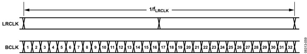
Figure 61. Example: 32 BCLK Cycles per Frame
