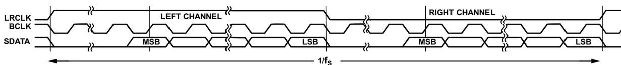
Figure 49. Right-Justified Mode—16 Bits to 24 Bits per Channel
