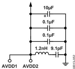
Figure 54. GSM Filter on the Analog Supply Pins
