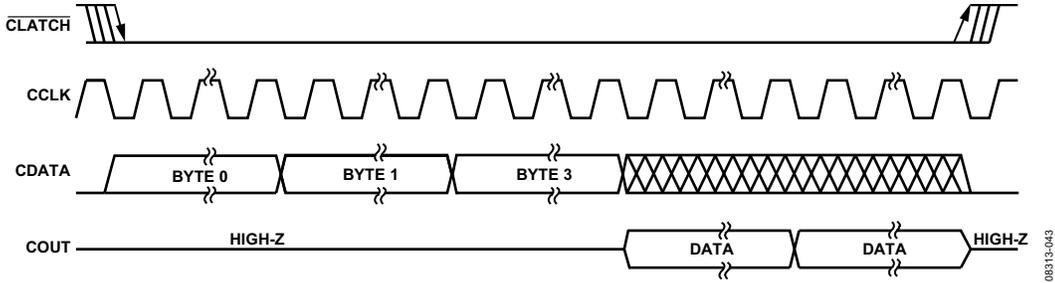
Figure 45. SPI Read from ADAU1381 Clocking (Single-Read Mode)
