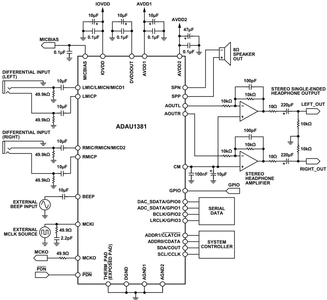
Figure 23. System Block Diagram with Differential Inputs
