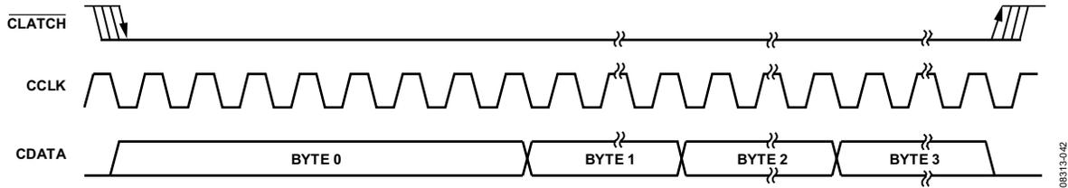
Figure 44. SPI Write to ADAU1381 Clocking (Single-Write Mode)
