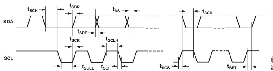
Figure 5. I<sup>2</sup>C Port Timing
