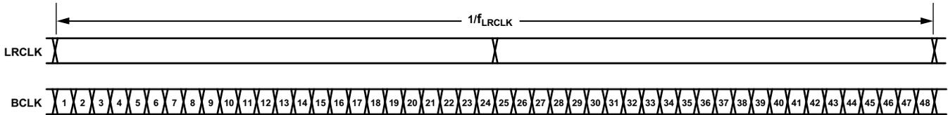
Figure 62. Example: 48 BCLK Cycles per Frame
