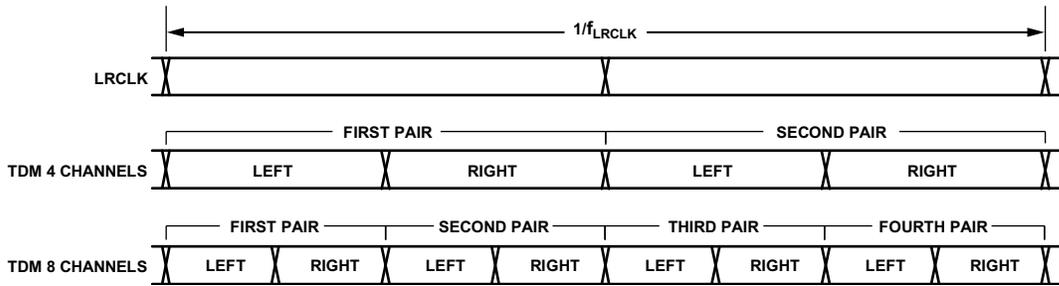
Figure 63. Left First Channel Selection in TDM
