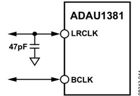
*Figure 46. TDM Pulse Mode LRCLK Capacitor Alignment*
