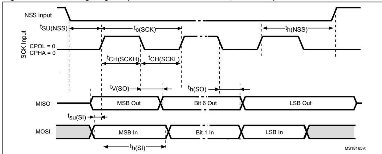
Figure 13. SPI timing diagram (Slave mode and CPOL = 1, CPHA = 1)
