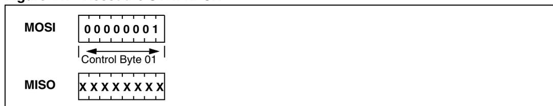
To reset the STRFNFCA using the SPI, the application sends the SPI Reset command (Control Byte 01, see [Figure 11](#)) which starts the internal controller reset process and puts the STRFNFCA into Power-up state. The STRFNFCA will wake up when pin  $\overline{IRQ\_IN}$  goes low. The STRFNFCA reset process only starts when the SPI\_SS pin returns to high level.
