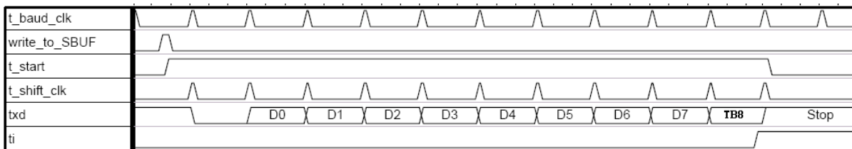
Fig. 7-5: Transmit modes 2 and 3 for Serial 0
