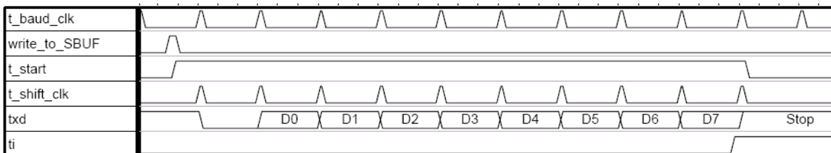
Fig. 7-3: Transmit mode 1 for Serial 0
