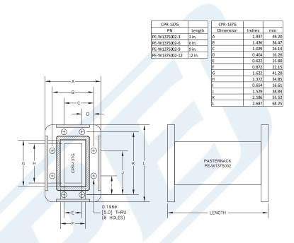
WR-137 Commercial Grade Straight Waveguide Section 12 Inch Length with CPR-137G Flange Operating from 5.85 GHz to 8.2 GHz from Pasternack Enterprises has same day shipment for domestic and International orders. Our RF, microwave and millimeter wave products maintain a 99% availability and are part of the broadest selection in the industry.
