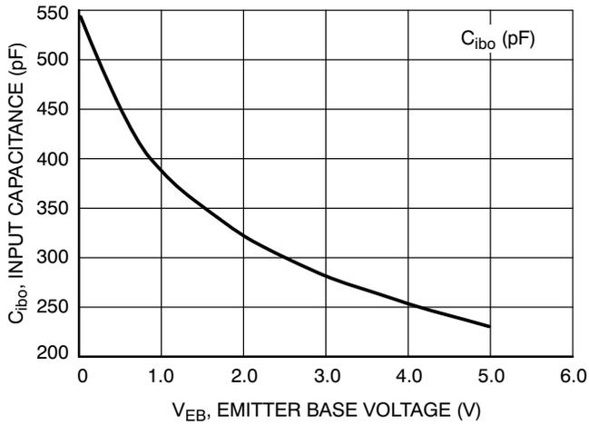
**Figure 7. Input Capacitance**
