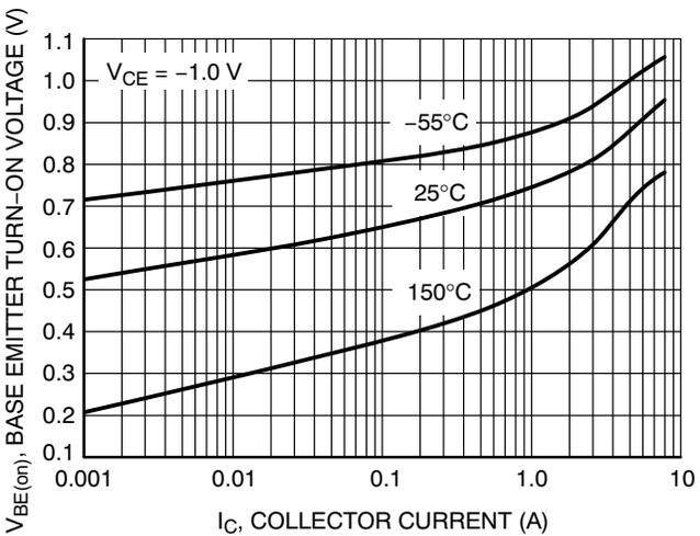
Figure 5. Base Emitter Turn-On Voltage vs. Collector Current
