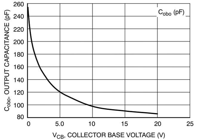
**Figure 8. Output Capacitance**
