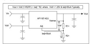
The AP1187 keeps a constant 1.25V between the VSENSE pin and the ADJ pin. By placing a resistor R1 across these two pins and connecting the VSENSE and VOUT pin together, a constant current flows through R1, adding to the IADJ current and into the R2 resistor producing a voltage equal to the (1.25/R1)\*R2 + IADJ\*R2. This voltage is then added to the 1.25V to set the output voltage. This is summarized in the above equation.
