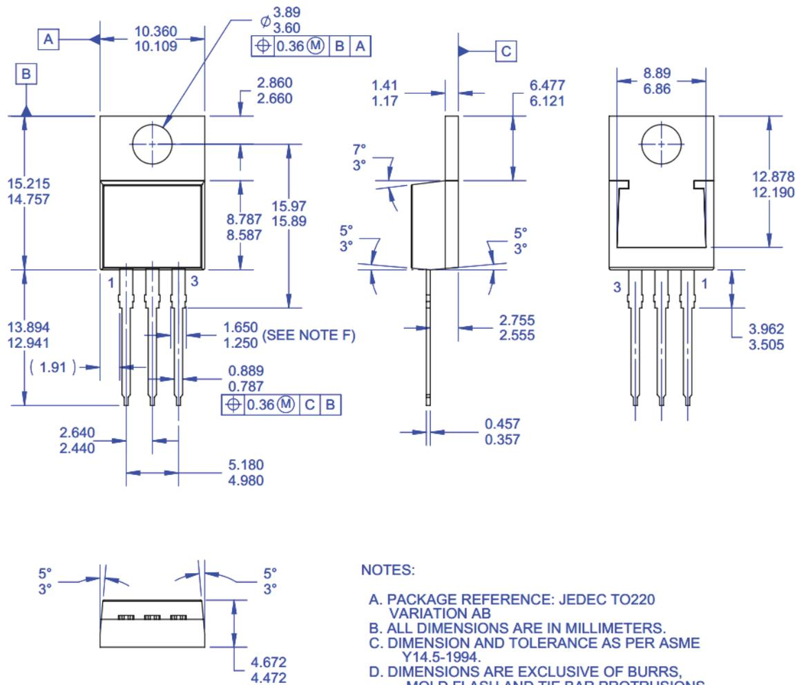
**Figure 16. TO-220, Molded, 3-Lead, Jedec Variation AB (Delta)**
