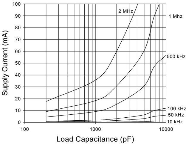
**Fig. 12 Supply Current vs. Frequency**
