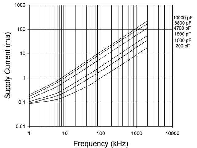
**Fig. 13 Supply Current vs. Load Capacitance**
