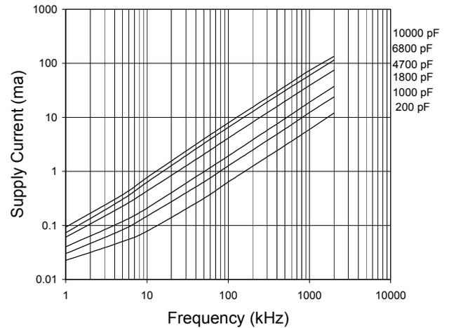
**Fig. 11 Supply Current vs. Load Capacitance**
