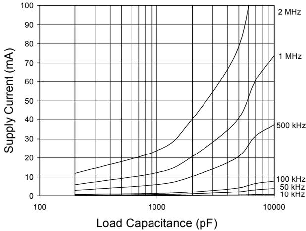
**Fig. 10 Supply Current vs. Frequency**
