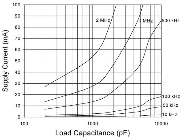
**Fig. 14 Supply Current vs. Frequency**
