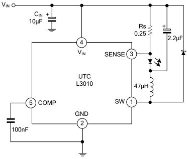
4.5~40V input voltage, 350mA output LED driver
