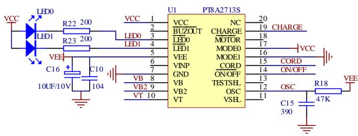
**Tact Switch Mode(Zero Delta Voltage Detection) of 2713**
