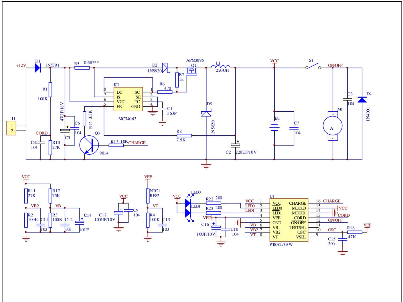
Slide Switch Mode(Zero Delta Voltage Detection) of 2713
