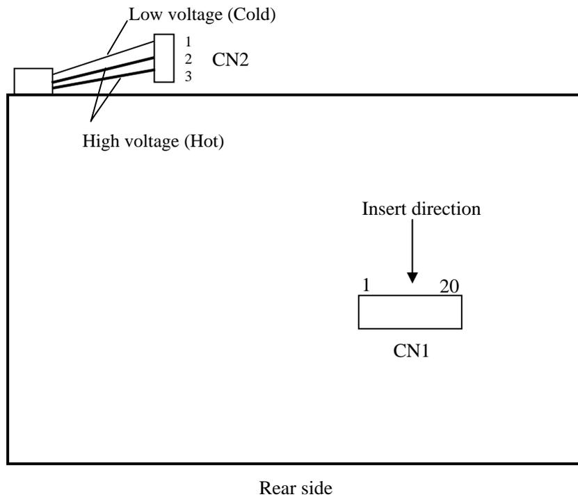
4.5.4 Connection between receiver and transmitter for LVDS
