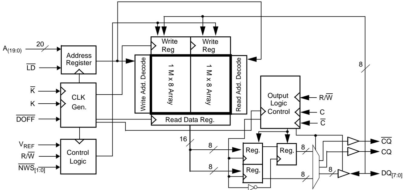
Logic Block Diagram (CY7C1916KV18)
