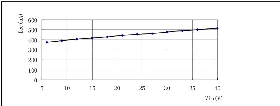
**Figure 1.2** ZLED7x20 Supply Quiescent Shutdown Current vs. Input Supply Voltage ( $V_{IN} = 6$  to 40 V)
