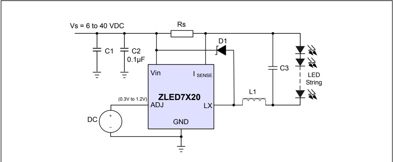
**Figure 3.3 Basic ZLED7x20 Application Circuit with Output Current Set by External Square Wave Voltage (PWM)**
