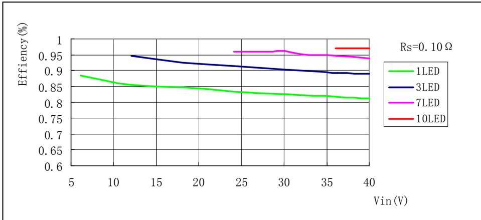
**Figure 1.4** Efficiency vs. Input Supply Voltage ( $V_{IN} = 6$  to  $40$  V)<sup>†</sup> Per Number of LEDs ( $R_s=0.15\Omega$ ,  $L_1=47\mu\text{H}$ )
