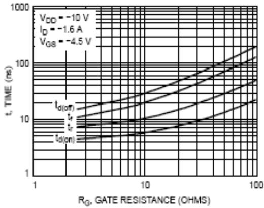
**Fig.7 Resistive Switching Time Variation vs. Gate Resistance**
