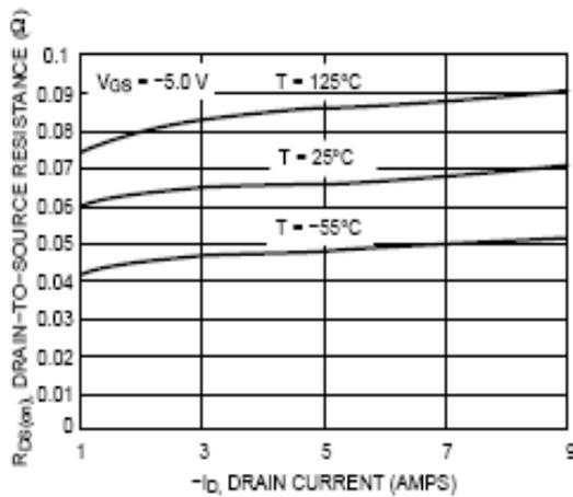
**Fig.3 On-Resistance vs. Drain Current and Temperature**
