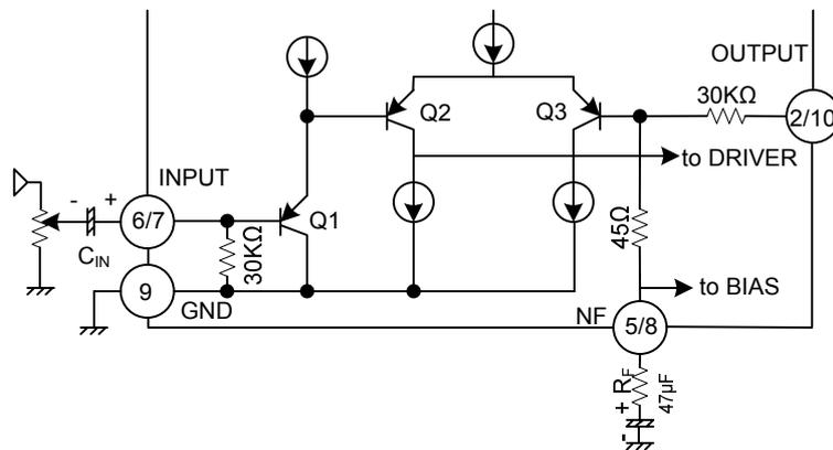
It is possible that without input coupling capacitor in the input circuit by use a PNP Transistor, Q1. However, 60mV max offset voltage is produced at pin (6) and (7). Application after checking volume slide noise is recommended. In order to cut the volume slide noise, insert the input capacitor ( $C_{IN}$ ) in series to interrupt the DC component.
