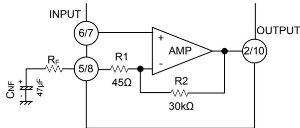
$$G_V = 20 \log \frac{R_F + R_1 + R_2}{R_F + R_1}$$
