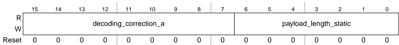
Figure 13-84. Protocol Configuration Register 19 (PCR19)
