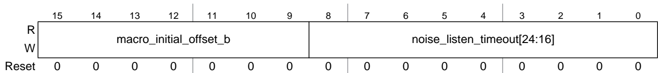
Figure 13-81. Protocol Configuration Register 16 (PCR16)
