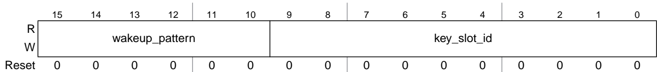
Figure 13-83. Protocol Configuration Register 18 (PCR18)
