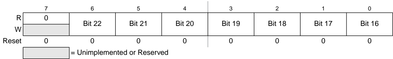
Figure 16-15. Debug Comparator Address High Register (DBGXAH)
