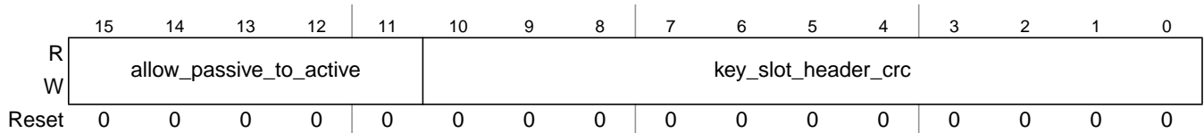
Figure 13-77. Protocol Configuration Register 12 (PCR12)
