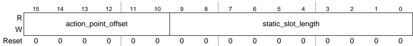
Figure 13-65. Protocol Configuration Register 0 (PCR0)
