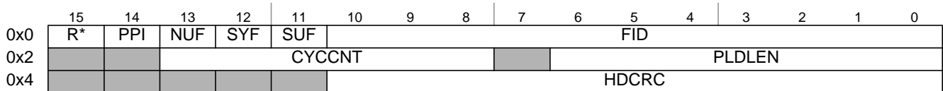
Figure 13-105. Frame Header Structure
