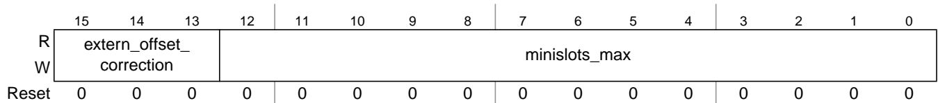
Figure 13-94. Protocol Configuration Register 29 (PCR29)
