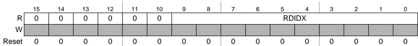
Figure 13-56. Receive FIFO B Read Index Register (RFBRIR)
