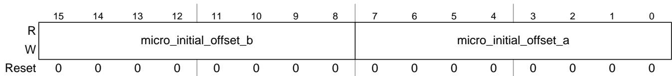
Figure 13-85. Protocol Configuration Register 20 (PCR20)
