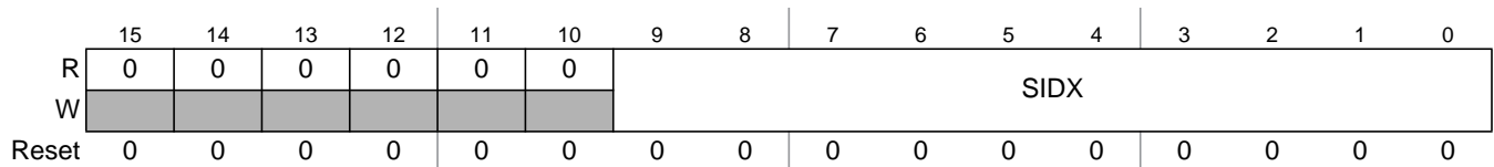
Figure 13-53. Receive FIFO Start Index Register (RFSIR)
