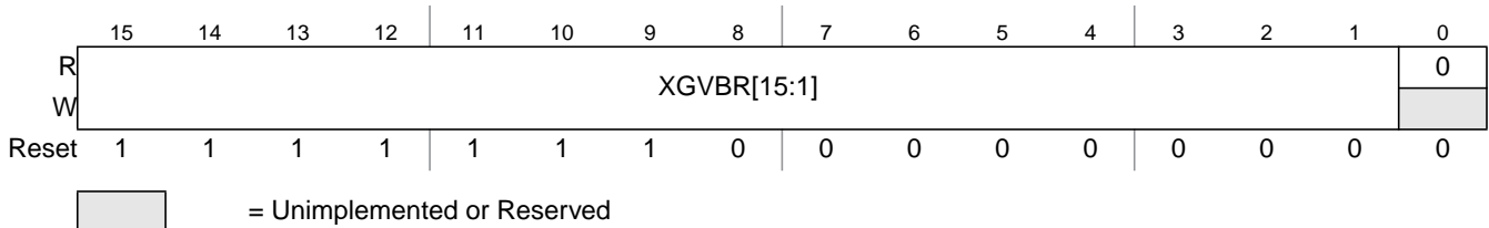
Figure 14-9. XGATE Vector Base Address Register (XGVBR)
