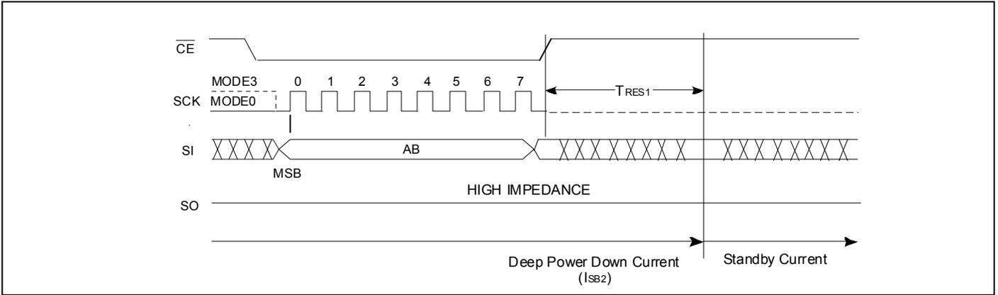
Figure 25: Release from Deep Power Down (RDP) Instruction
