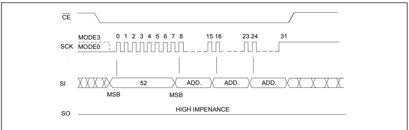
Figure 14: 32K-byte Block Erase Sequence
