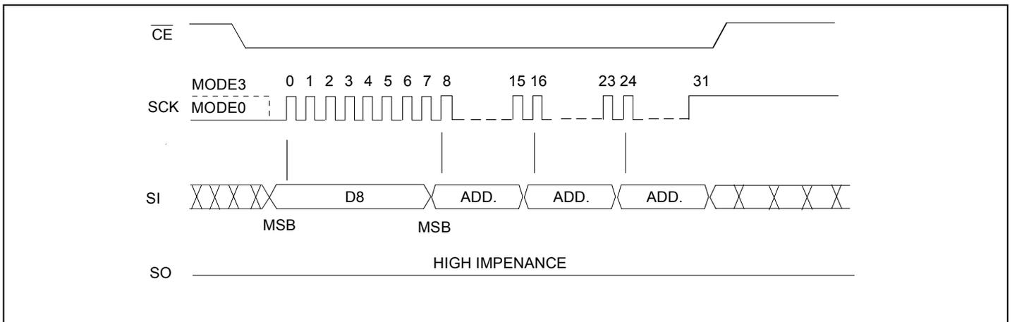
Figure 13: 64K-byte Block Erase Sequence
