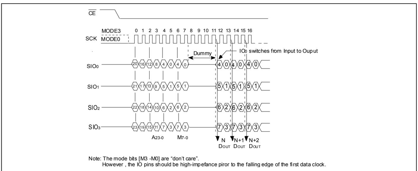
Figure 9: Fast Read Quad I/O Sequence ([M<sub>7</sub>-M<sub>0</sub>] = AxH)
