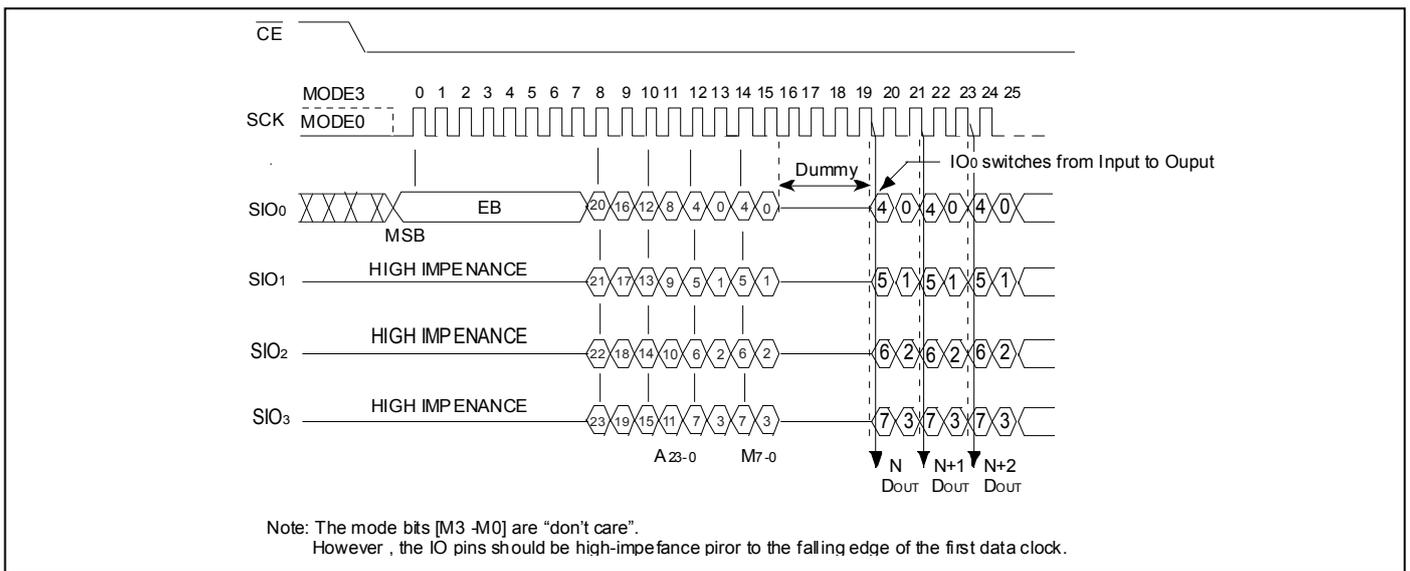
Figure 8: Fast Read Quad I/O Sequence ([M<sub>7</sub>-M<sub>0</sub>] = 0xH or NOT AxH)
