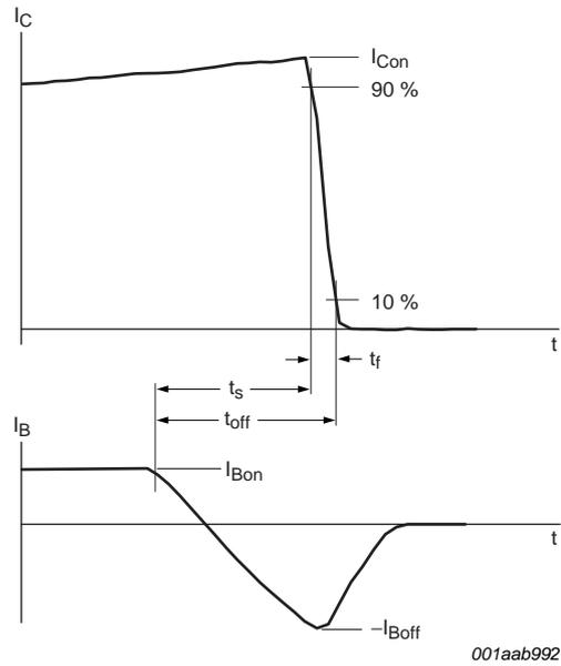
**Fig 15. Switching times waveforms for inductive load**
