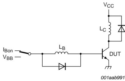
$V_{BB} = -5\text{ V}; L_C = 200\ \mu\text{H}; L_B = 1\ \mu\text{H}$
