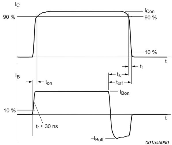
**Fig 13. Switching times waveforms for resistive load**
