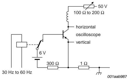
**Fig 6. Test circuit for collector-emitter sustaining voltage**
