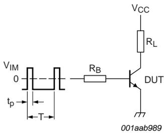
$V_{IM} = -6 \text{ to } +8\text{V}; t_p = 20\text{ }\mu\text{s}; \delta = \frac{t_p}{T} = 0.01$
