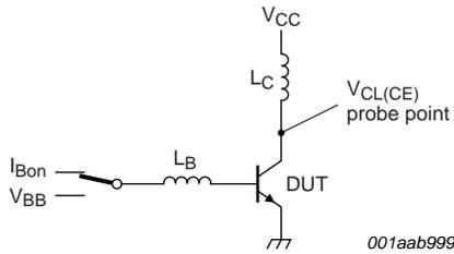
$V_{CL(CE)} \leq 1000 \text{ V}; V_{CC} = 150 \text{ V}; V_{BB} = -5 \text{ V};$
