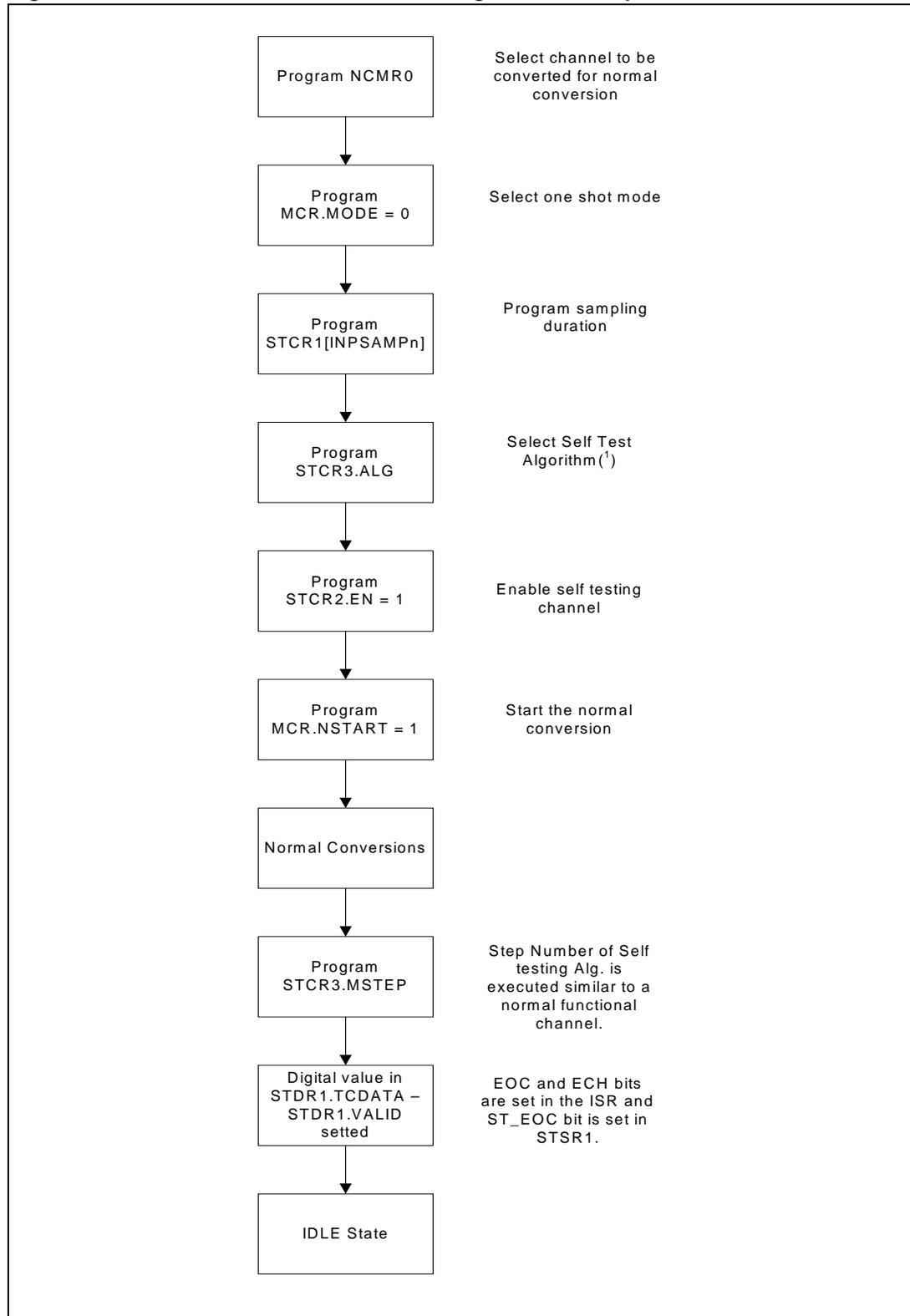
1. In one shot mode, if test channel is enabled, only one step of selected self testing algorithm is executed at the end of the chain. The step number and algorithm to be executed is programmed in STCR3 register.
