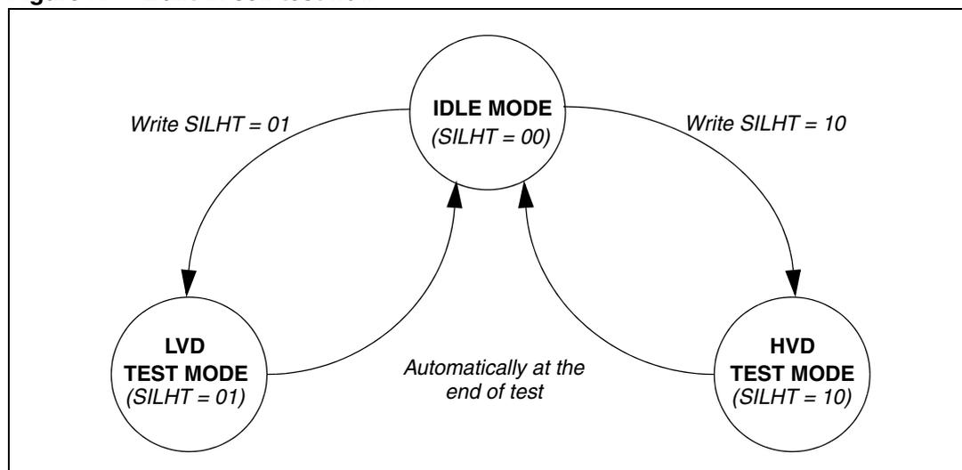
Figure 8. PMU power-on self test flow
