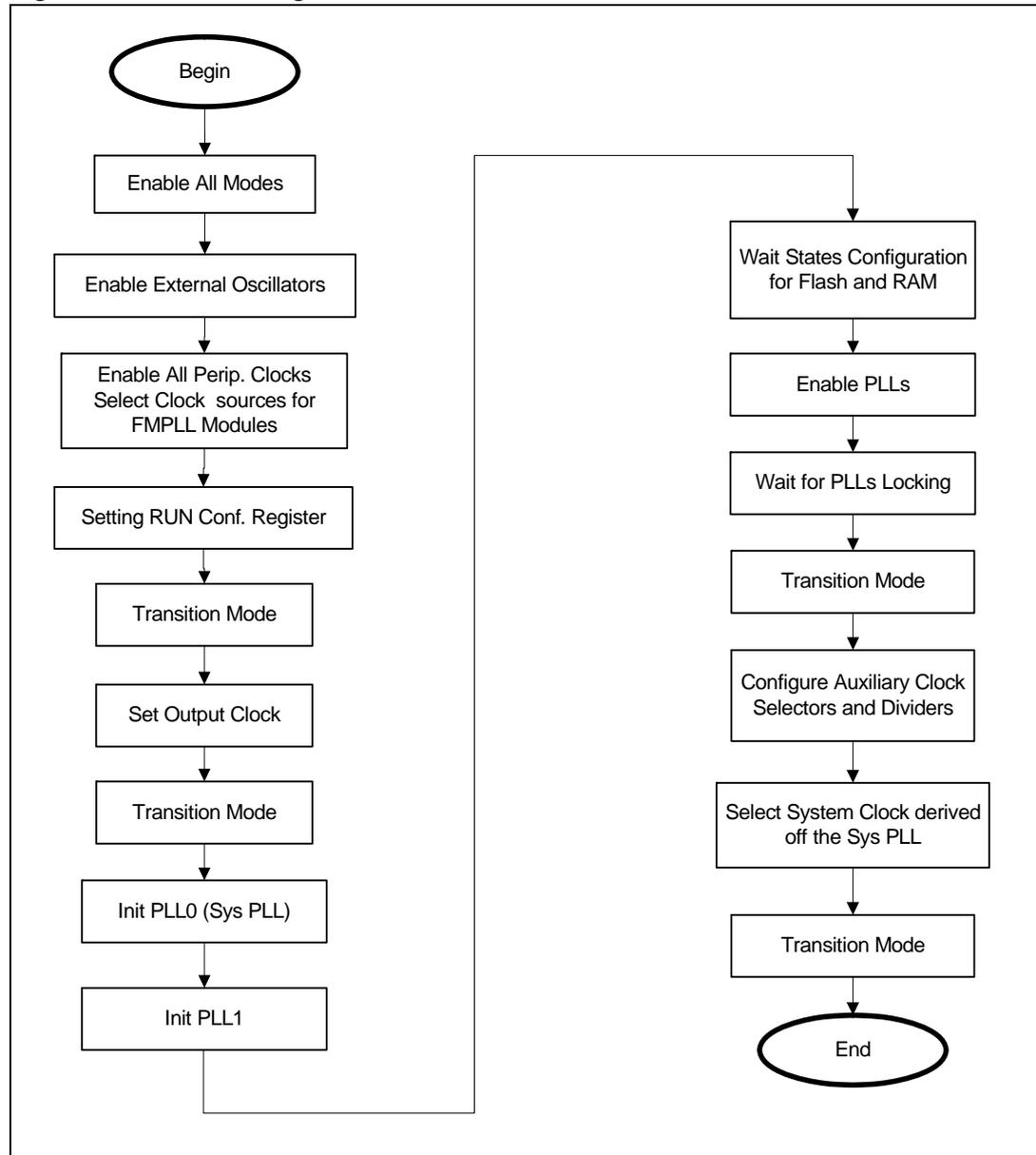
c. Flash and SRAM wait states depend on MCU work frequency. For this reason it's a good choice to configure these together with clocks.
