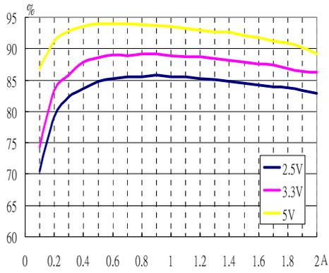
**Figure 7 Efficiency (V<sub>IN</sub>=7V)**
