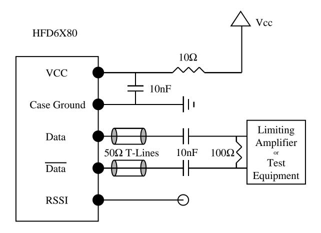
The 100 $\Omega$  resistor prior to the limiting amplifier is needed only when the input impedance of the amplifier is not 50 $\Omega$  DC blocking capacitors must also be present at the TIA outputs to avoid a large DC current which may damage the chip.
