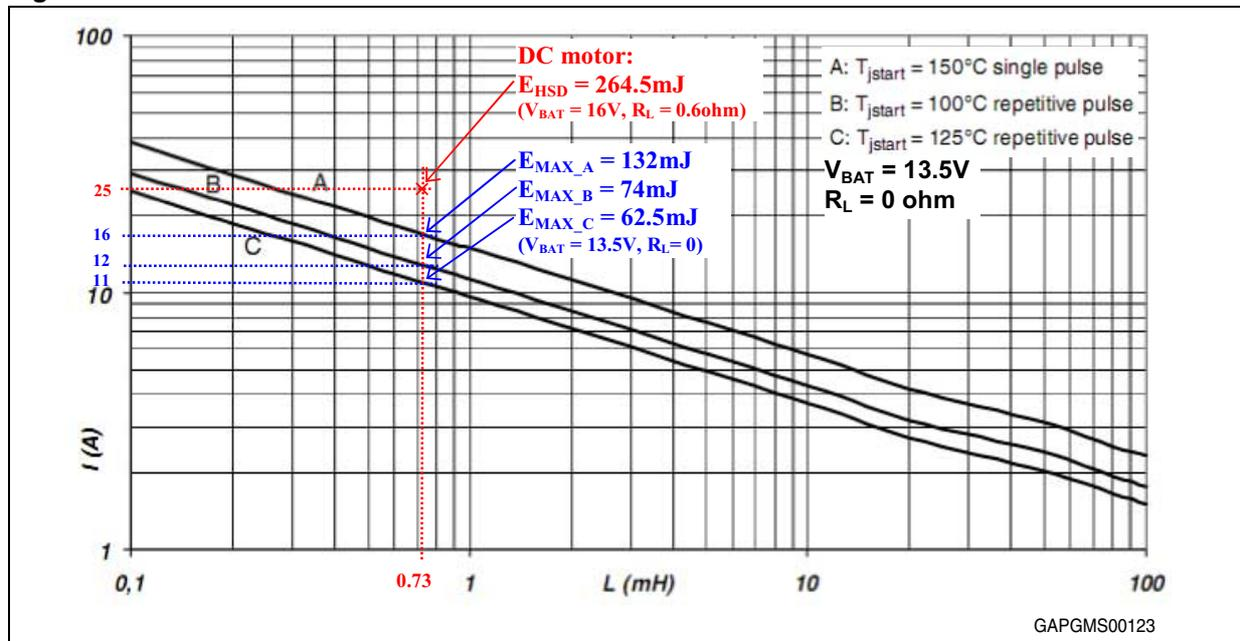
The demagnetization energy is by a factor of 2 higher than the device is able to withstand, therefore additional protection/clamping is necessary.
