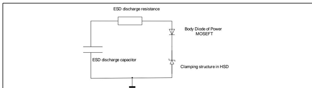
A positive ESD pulse on the output is transferred through the body diode of the power MOSFET to the Vcc pin of the HSD, stressing the Vcc-GND clamping structure. The ESD ratings of the Vcc-GND clamping structure is the same for the output clamping structure.
