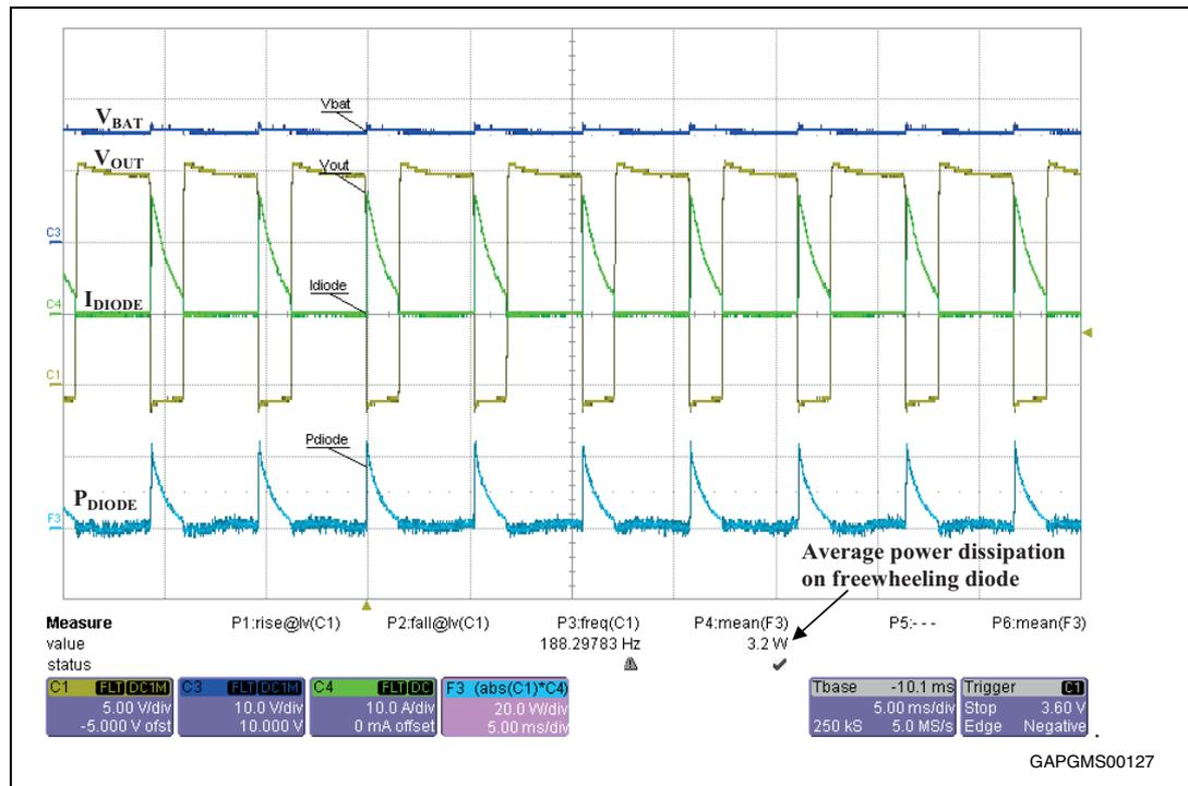
The average power dissipation measured on the freewheeling diode is 3.2 W, while the HSD thermal shutdown cycling frequency was 188 Hz. These values are below theoretical calculations. Real HSD cycling frequency is much lower than the frequency assumed in the calculation (500 Hz – based on simulation with resistive load).
