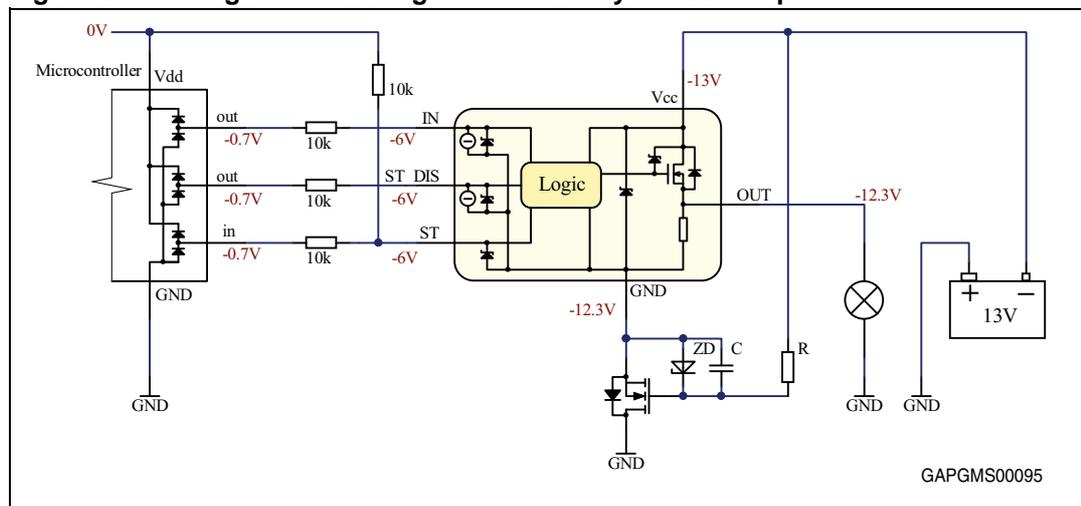
The HSD is protected by a MOSFET which is switched-off during reverse battery conditions. This MOSFET circuitry also provides full ISO pulse clamping at supply line and causes no ground level shift. A capacitor between gate and source keeps the gate charged during negative ISO pulses as well. The time constant given by RC values should be longer than 2 ms (duration of reverse battery protection (monolithic HSDs only) - comparison of negative ISO7637 pulse 1).
