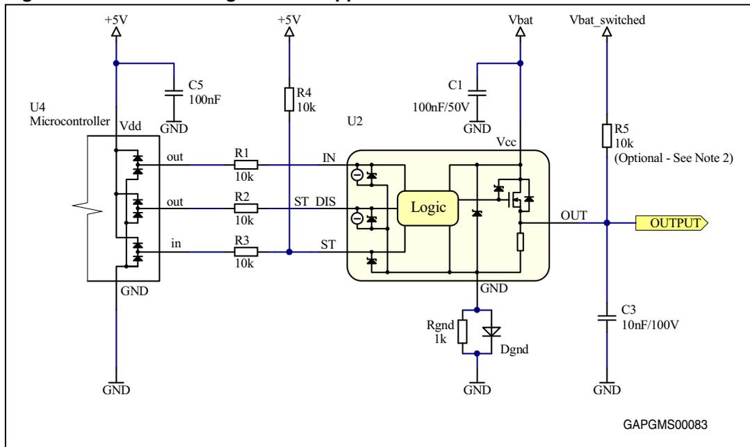
1. If status disable function is not required, ST\_DIS pin should be left open or connected to ground through a resistor (~10 kΩ). Direct connection to ground is not safe (ISO pulses clamped through ST\_DIS pin can damage the device).
