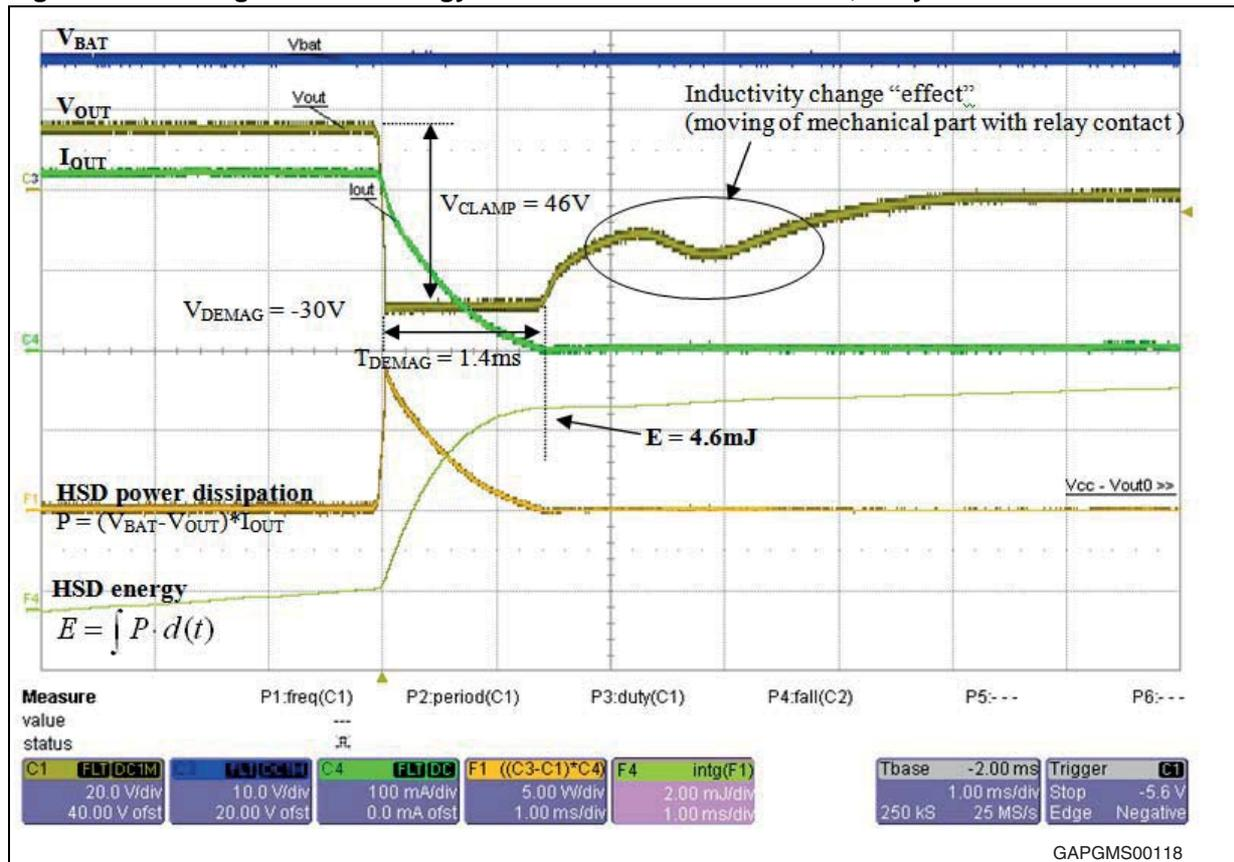
The measured energy is lower by a factor of two than calculated (4.6 mJ measured versus 9.9 mJ calculated). This difference can be explained by measurement at ambient temperature when the coil resistance is ~25 % higher than the resistance at -40 °C used in the calculations. Another factor is the coil inductance decrease due to the magnetic saturation (the inductance value used for calculation was measured at a low current).
