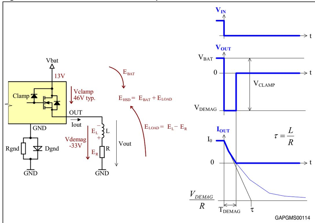
The HSD turn-off phase with inductive load is explained in [Figure 37](#). The inductance reverses the output voltage in order to be able to continue the current in the same
