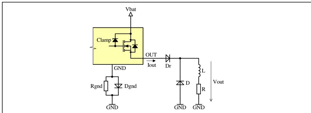
A general purpose diode connected in parallel with the load provides a conductive path for proper demagnetization. Relatively small demagnetization voltage (1 diode voltage drop in forward direction) leads to a very slow demagnetization. This can have a negative influence when driving the relay, for example. A slow movement of the armature (slow opening of contacts) can have a negative influence on the lifetime of the relay contacts (depending on the switching current).
