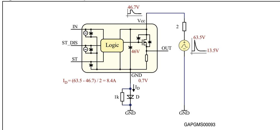
The most severe negative ISO pulse to consider is test pulse 1 at level IV (-100 V@2 ms). This pulse is directly transferred to the GND pin. The maximum peak reverse voltage of the diode should therefore be at least 100 V.
