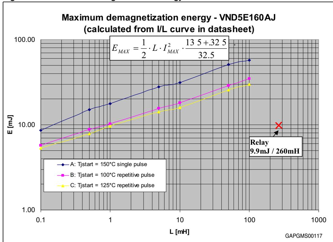
Waveform A represents the max energy the device can withstand in a single pulse. A second pulse with the same energy can destroy the part. Waveforms B and C represent the max energy to ensure the junction temperature variation to stay below 60 K.
