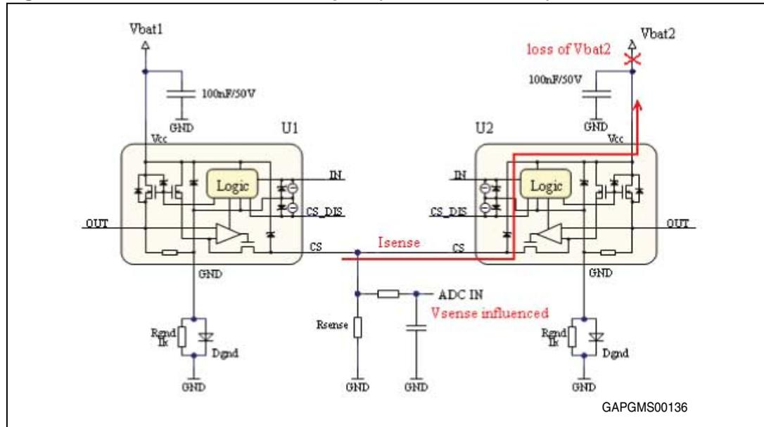
Direct connection of CS pins is not safe in following cases:
