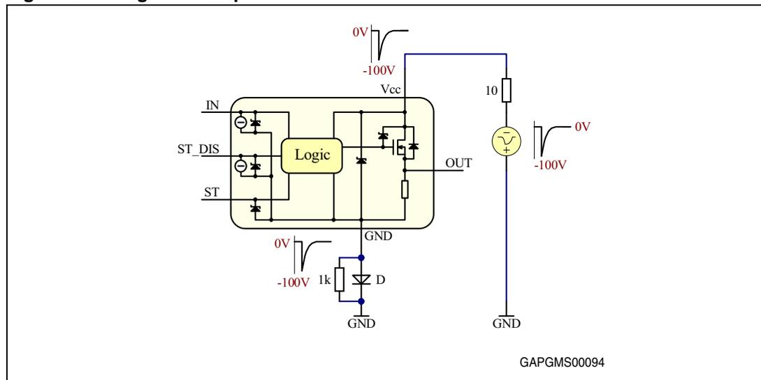
*Note:* As seen from the above explanation, the HSD with diode protection in the GND pin doesn't clamp negative ISO pulses at supply line. Therefore an appropriate serial protection resistor should be used between the  $\mu$ C and HSD. The resistor value should be calculated according to maximum injected current to the I/O pin of the used microcontroller.
