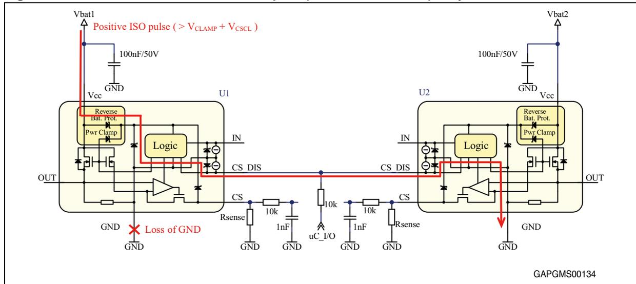
Direct connection of CS pins is not safe in the following cases:
