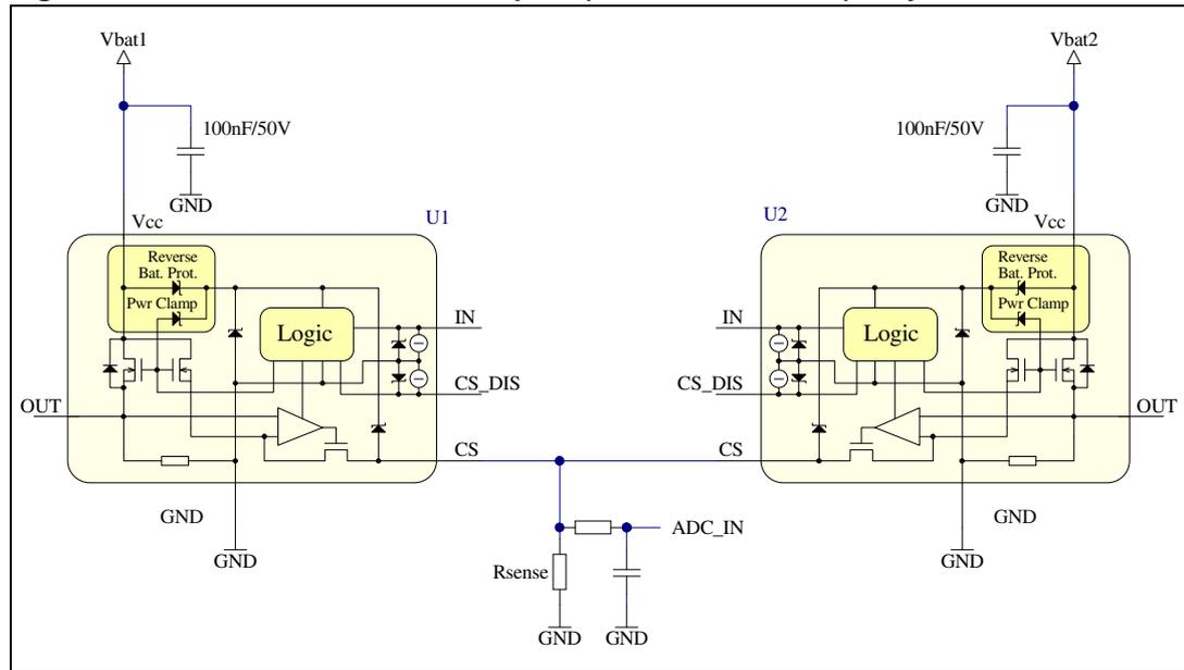
Direct connection of CS pins is not safe in following cases:
