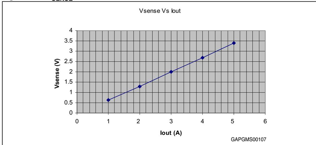
The trend is almost linear in the application range and so we can approximate the  $V_{SENSE}$  trend with the following equation:
