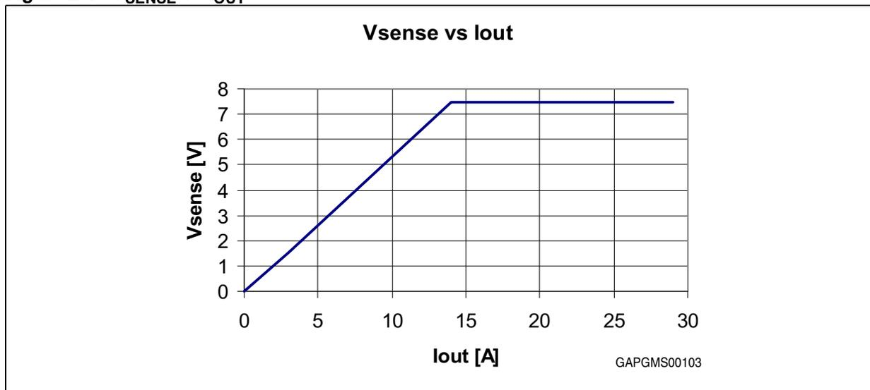
On the other hand, care must be taken to prevent the P channel MOSFET M1 from saturation, causing the  $I_{SENSE}$  to again be disproportional with  $I_{OUT}$ . This normally happens when the maximum current that M1 is able to supply is reached ( $11\text{ mA typ.}$ )
