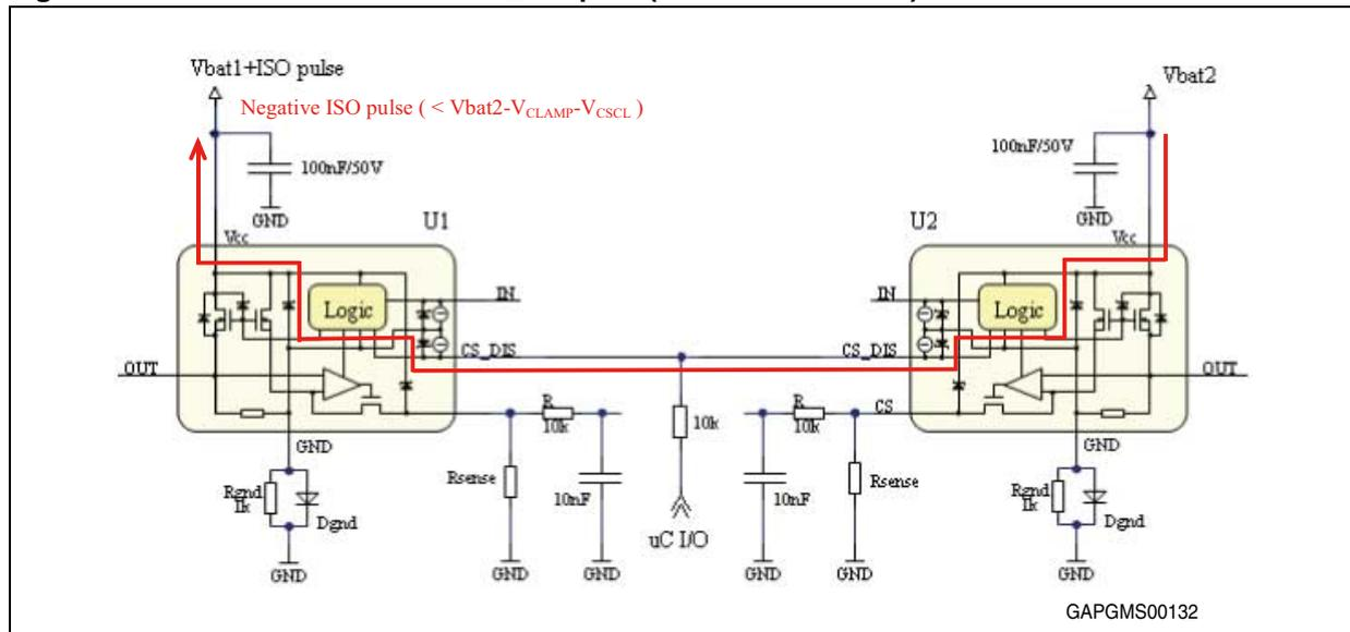
Direct connection of CS\_DIS pins is not safe in following cases:
