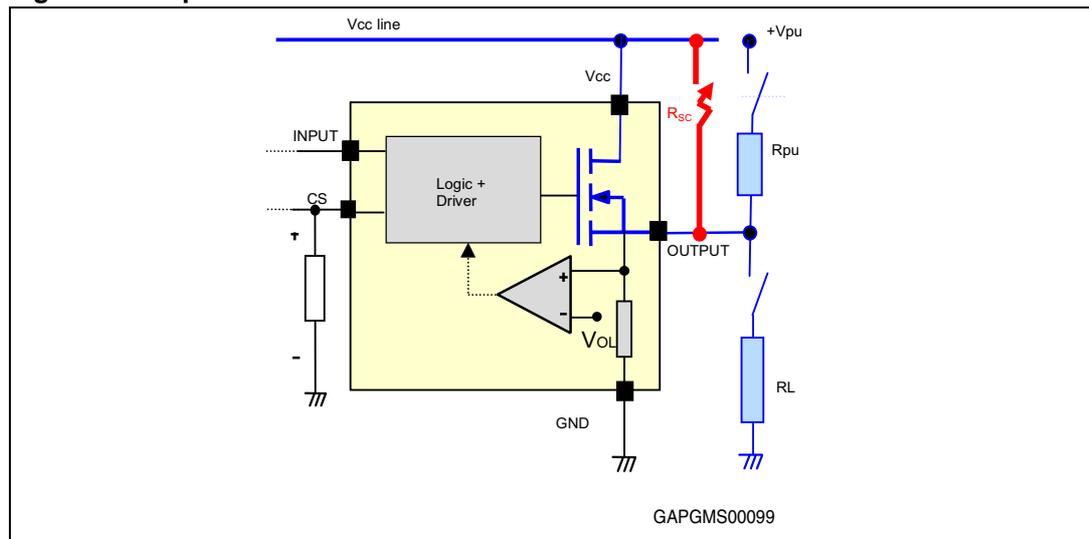
Figure 14. Open load/short to Vcc condition
