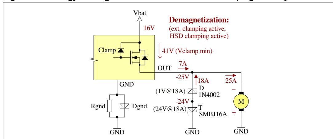
The output voltage during the demagnetization phase is -25 V (considering a worst case HSD  $V_{ClampMin} = 41\text{ V}$ ,  $V_{BAT} = 16\text{ V}$ ).
