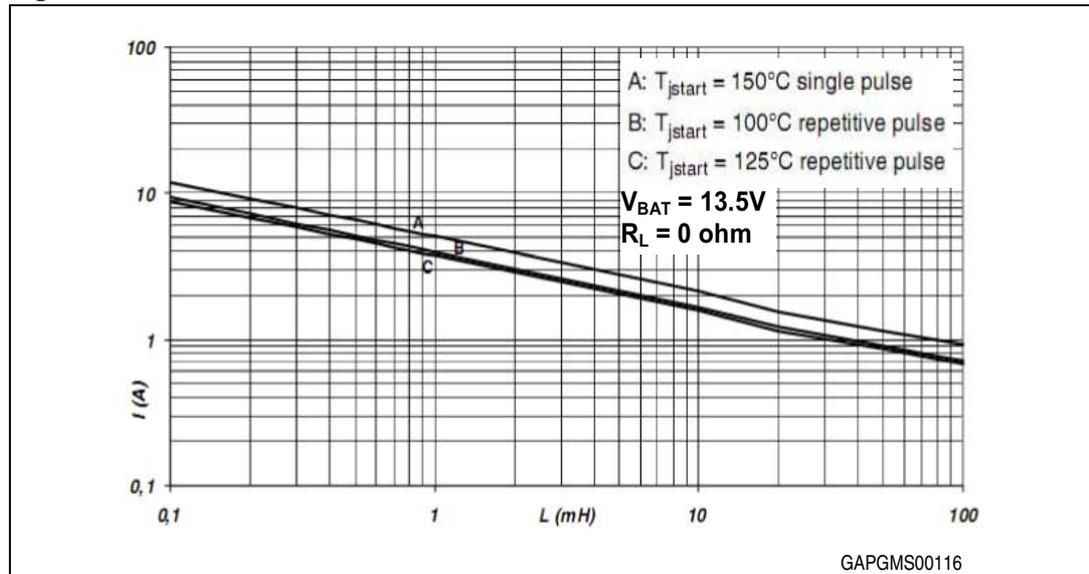
Therefore it is convenient to translate I/L chart to E/L chart. This can be easily done using Equation 15 for the calculation of energy on the HSD considering  $R_L = 0$ ,  $V_{BAT} = 13.5\text{ V}$  (see Figure 40).
