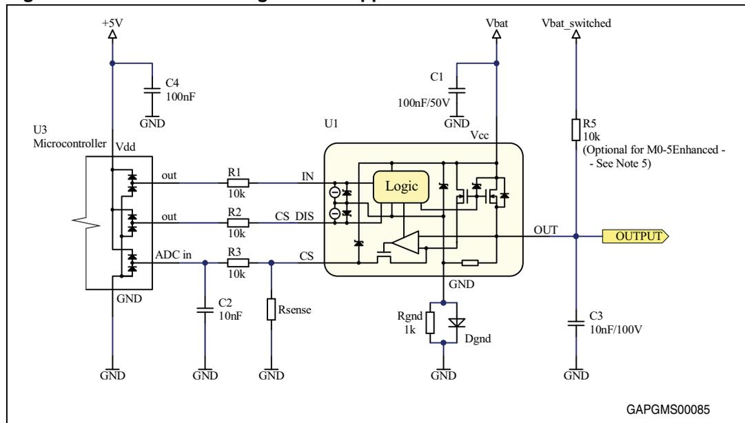
**Figure 3. Hybrid analogue HSD – application schematic**
