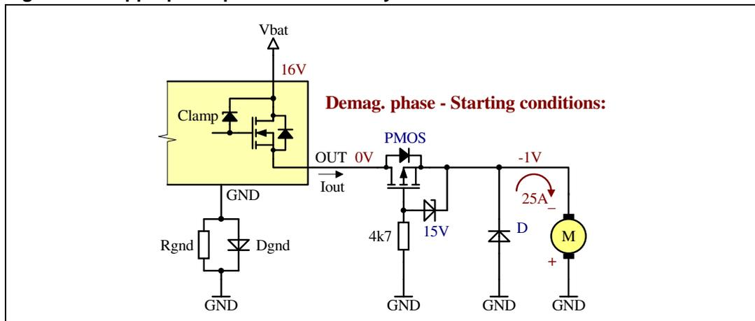
Demagnetization time - Equation 12 (Assuming  $V_{DEMAG} = -1 \text{ V}$ ) :
