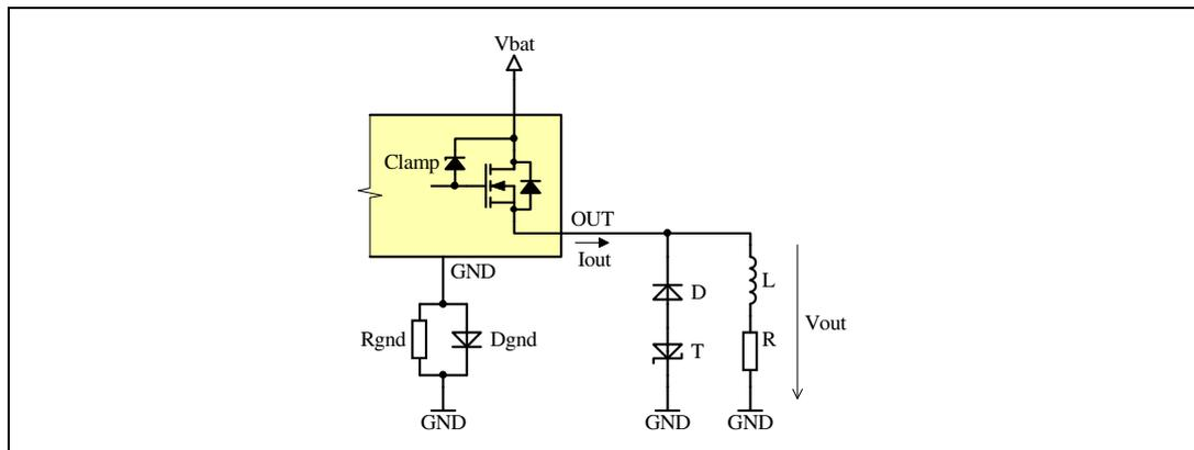
The transil (T) clamps the demagnetization voltage to a safe level. The clamping voltage of the transil should be selected in a way that the voltage across the HSD channel is below the minimum specified clamping voltage of the HSD (41 V). The diode (D) is included to protect the transil during normal operation (positive output voltage).
