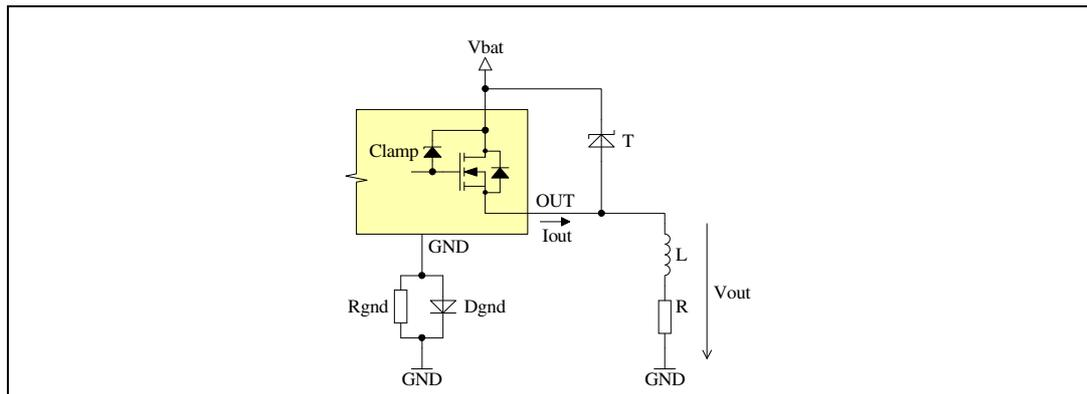
The HSD channel is protected directly by the parallel transistor. The clamping voltage of the transistor should be below the minimum clamping voltage of the HSD (41 V). Such transistors ( $V_{CL} < 41 \text{ V}$ ) usually start conducting at 30 V, therefore there is a high probability that it is damaged during the clamped load dump pulse (36 V). For that reason it is usually better to use the previously described solution (1).
