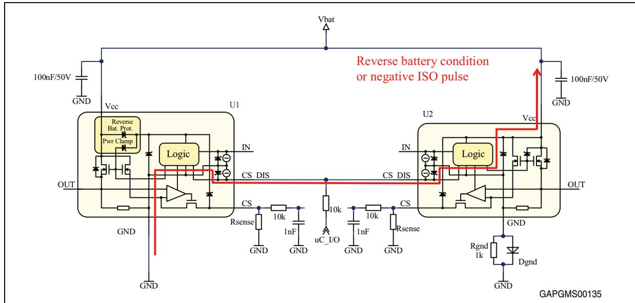
Direct connection of CS pins is not safe in the following cases (single supply line considered):
