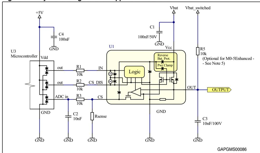
4. If current sense disable function is not required, CS\_DIS pin should be left open or connected to ground through a resistor (~10 kΩ). Direct connection to ground is not safe (ISO pulses clamped through CS\_DIS pin can damage the device).
