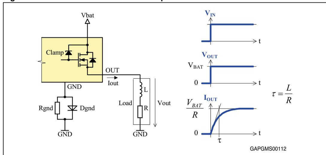
When an HSD turns on an inductive load, the current increases with a time constant given by  $L/R$  values, so the nominal load current is not reached immediately. This fact should be considered in diagnostics software (i.e. to avoid false open load detection).
