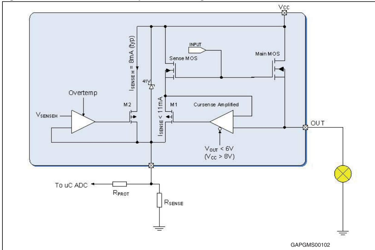
The SenseMOS is scaled down copy of the MainMOS according to a defined geometric ratio, driven by the same gate control circuit as the MainMOS.
