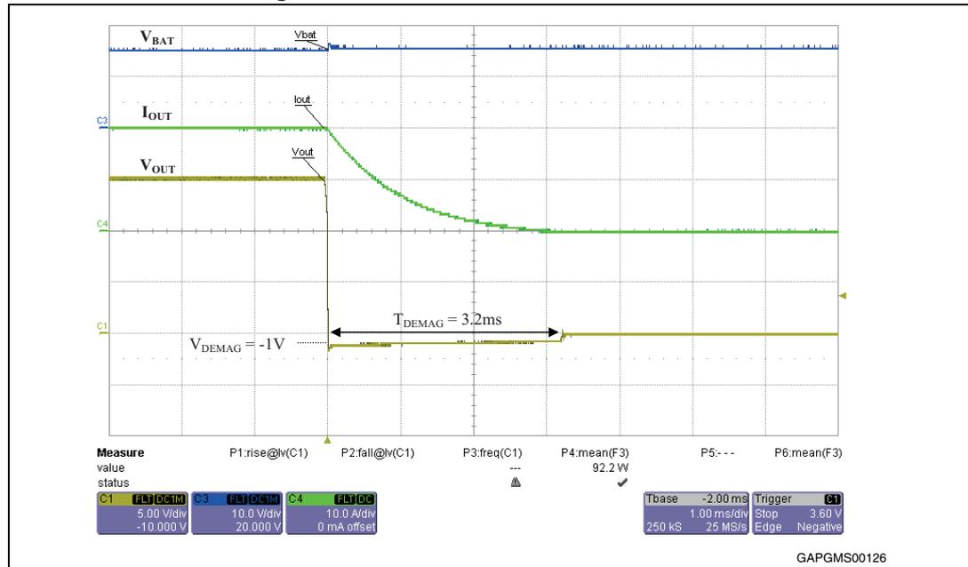
The measured demagnetization time of 3.2 ms is very close to the calculated value (3.37 ms). Due to the measurement at room temperature, the stall current was only 20 A (versus 25 A specified at -40 °C).
