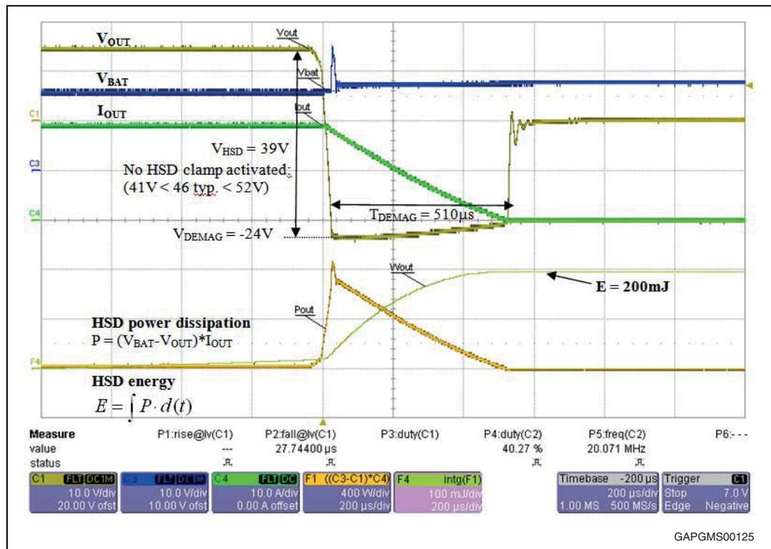
The measured energy is significantly lower than the calculated one (200 mJ measured versus 260 mJ calculated), while the demagnetization time fits well. This difference can be explained by measurement at ambient temperature when coil resistance is ~25 % higher than the resistance at -40 °C used in the calculations.
