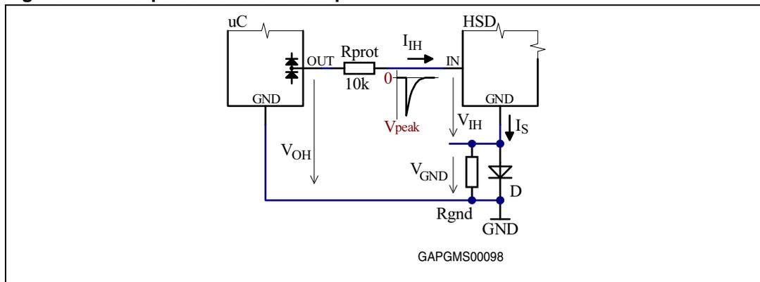
Therefore, each microcontroller I/O pin connected to a HSD must be protected by a serial resistor to limit the injected current. The value of  $R_{PROT}$  must be high enough to ensure that injected current is always below the latch-up limit of the microcontroller I/O. We should also consider the voltage drop on  $R_{PROT}$  because the current required by the HSD input is typically 10  $\mu$ A. The following condition must be fulfilled:
