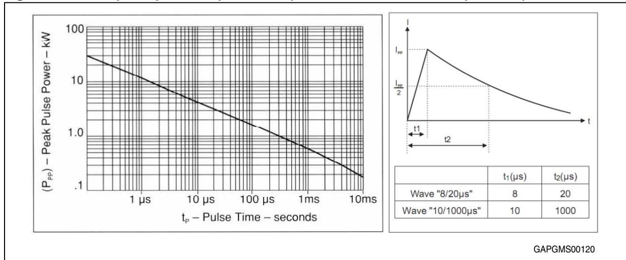
Figure 45. Equivalent pulses giving the same power dissipation
