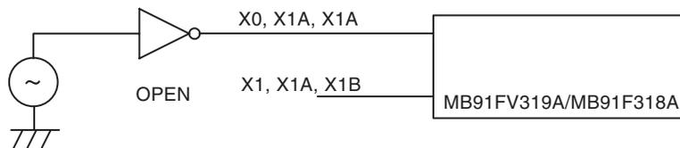
Note : The X1 (X1A, X1B) pin must be designed to have a delay within 15 ns, at 10 MHz, from the signal to the X0 (X0A, X0B) pin.
