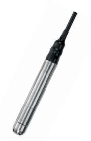
The ILTSU is designed for use in continuous submersion in liquids such as water, oil and fuels. The probe uses the latest piezoresistive media-isolated silicon sensing technology and a stainless steel diaphragm. Housed within a 316L stainless steel, or high grade Duplex stainless steel housing, this submersible transmitter is the ideal product for hydrostatic level measurement where temperature is also a critical part of the measurement.
