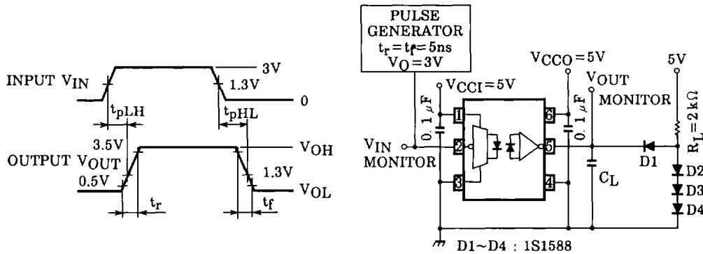
$C_L$  is approximately  $15\text{pF}$  which includes probe and stray wiring capacitance.
