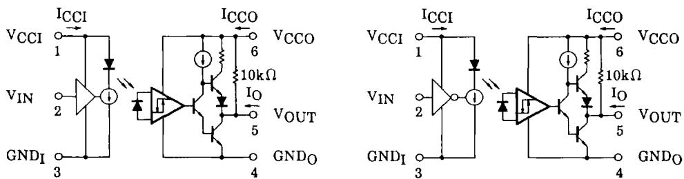
A  $0.1\mu\text{F}$  bypass capacitor must be connected between pin 1 and 3, and between pin 4 and 6.
