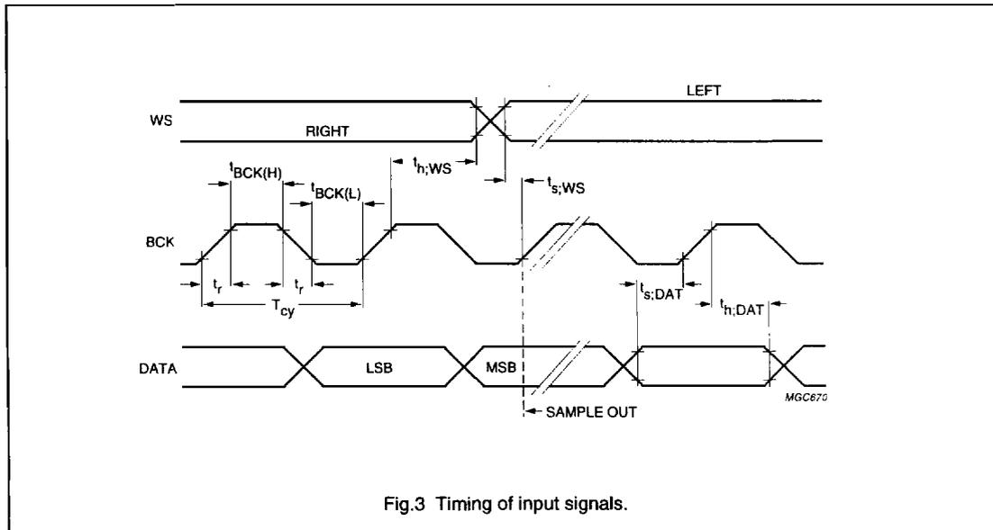
Fig.3 Timing of input signals.
