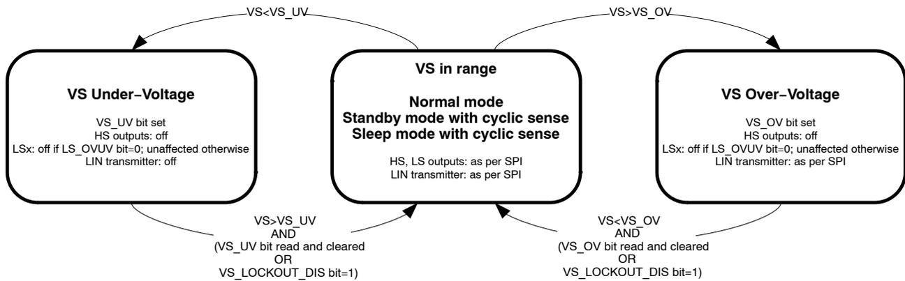
Figure 17. Under- and Over-voltage on VS Supply
