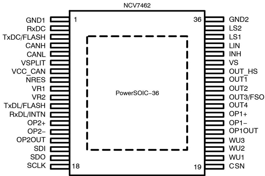
Figure 2. Package Pin-out
