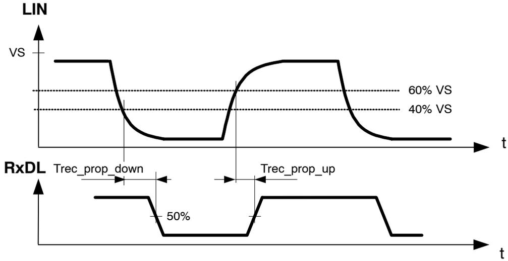
Figure 8. LIN Dynamic Characteristics - Receiver
