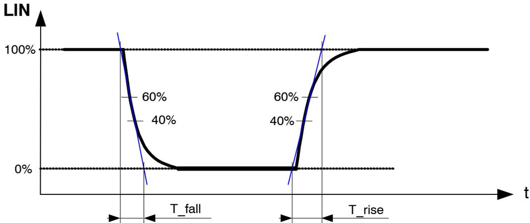
**Figure 7. LIN Dynamic Characteristics – Transmitter Slope**
