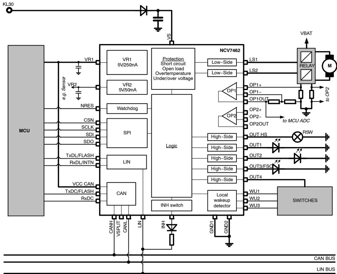
Figure 3. Application Diagram
