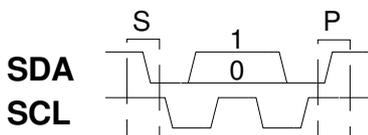
**Figure 3.** I<sup>2</sup>C<sup>®</sup> bus protocol definitions
