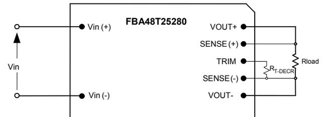
Figure 5. Configuration for decreasing output voltage.
