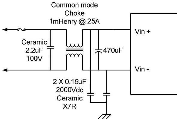
**Figure 6.** Input Filter Configuration Required to Meet CISPR 22 Class A for Conducted Emissions.
