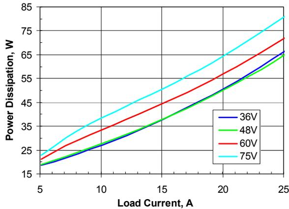
Figure 11. Power dissipation vs. load current and input voltage for FBA48T25280 converter at Ta = 25°C.
