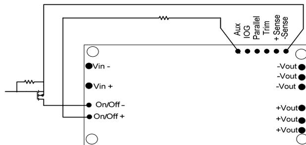
Figure 2. ON/OFF Control Using Auxiliary Voltage
