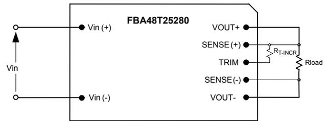
Figure 4. Configuration for increasing output voltage.
