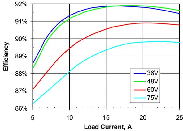
Figure 10. Efficiency vs. load current and input voltage for FBA48T25280 converter at Ta=25°C.
