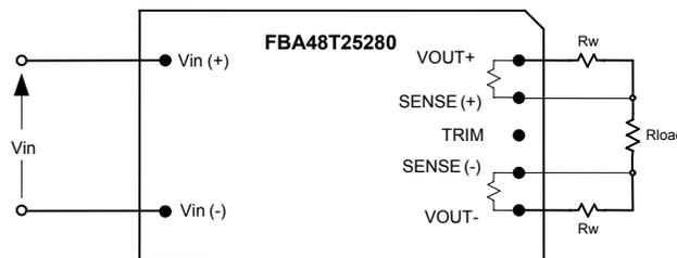
Figure 3. Remote sense circuit configuration.
