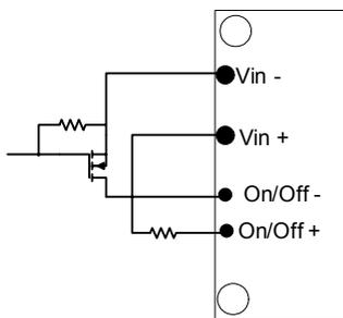
Figure 1. ON/OFF Control Using Vin
