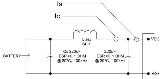
Figure 13. Test setup for measuring input reflected ripple currents, ic and is.
