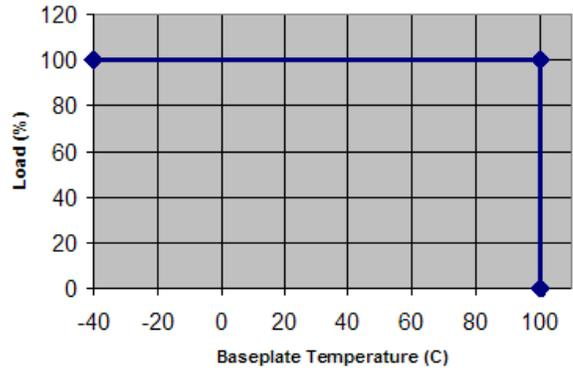
Figure 12. Available Power Vs. Baseplate Temperature
