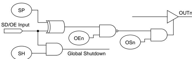
When configured as SD, device is shut down, and the single-ended LVCMOS outputs are driven low. When configured as OE, and outputs are disabled, the outputs are driven high/low.
