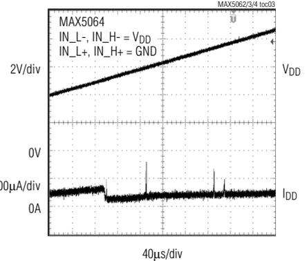
**$I_{DD} + I_{BSTO}$  vs.  $V_{DD}$
