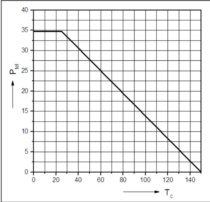
**Figure 1: Power dissipation**
