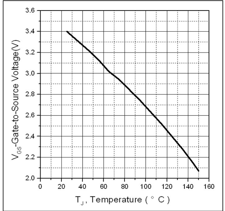
**Figure 2. Typ. Gate to source cut-off voltage**
