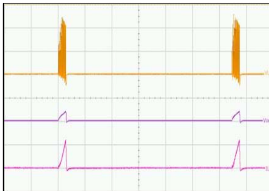
(VIN = 5 V, VOUT = 1.8 V, IOUT = Current Limit, no CSS) Upper Trace: LX Pin Voltage, 5 V / div Middle Trace: Output Voltage, 2 V / div Lower Trace: Inductor Current, 2 A / div Time = 500 \mu s / div
