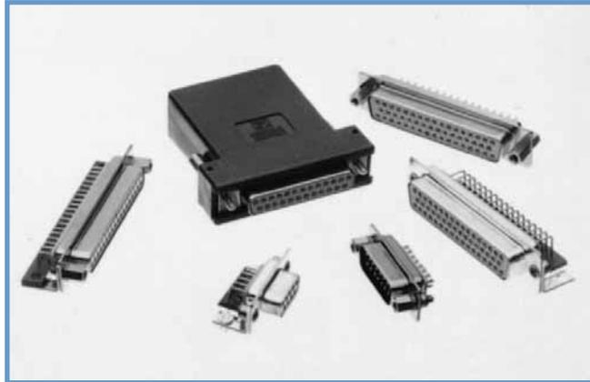
Harmo-D series connectors are military quality connectors designed for use in sheltered, mildly corrosive environments having a wide range of temperature, pressure and humidity changes. Applicable fixed contact connectors are qualified to MIL-DTL-24308 (see pages 84-94 for listing) and meet the performance requirements of IEC 60807-2, Performance Level One.
