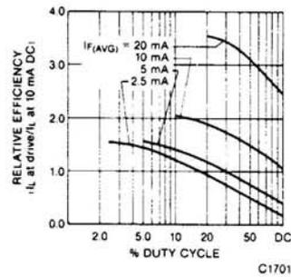
Fig. 5. Relative Efficiency vs. Duty Cycle
