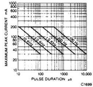
Fig. 3. Maximum Peak Current vs. Pulse Duration
