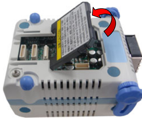
Figure 2-1. Acrylic Board Removal Method
