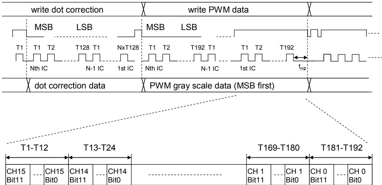
$t_{H2}$ : In the end of gray scale mode,  $DCLK -LE$  should be no less than 10ns.
