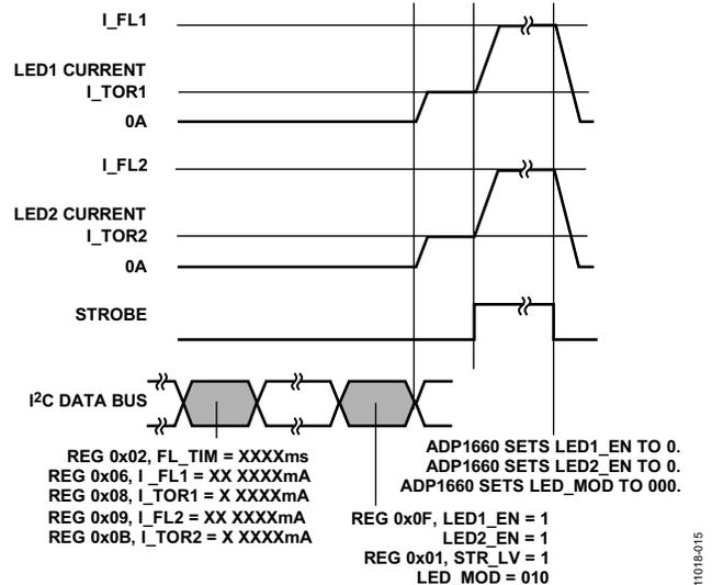
Figure 20. Enabling Assist to Flash (Level-Sensitive) Mode
