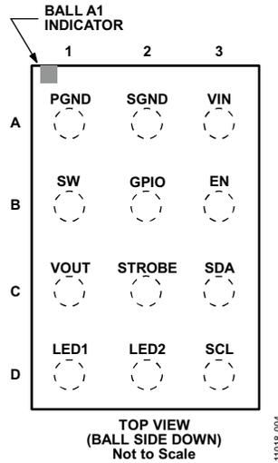
Figure 4. Pin Configuration
