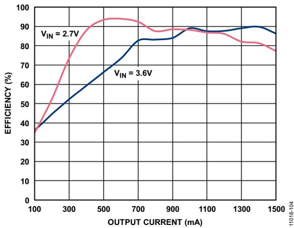
Figure 13. Efficiency ( $P_{LED}/P_{IN}$ ) vs. LED Output Current
