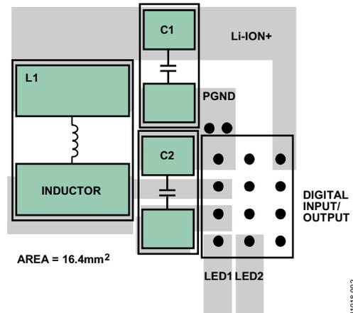
Figure 2. PCB Layout
