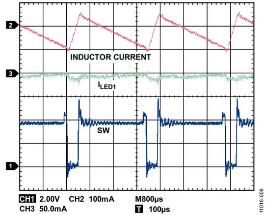
Figure 8. Switching Waveforms, Flash Mode,  $I_{LED1} = I_{LED2} = 750mA$
