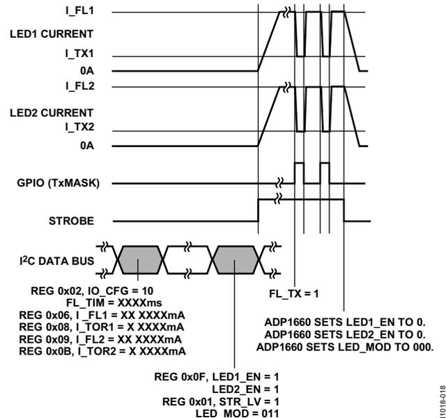
Figure 23. TxMASK Operation During Flash (Level-Sensitive) Mode
