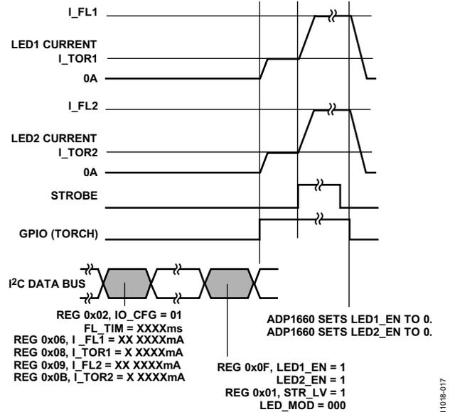
Figure 22. Enabling Flash Mode from External Torch Mode
