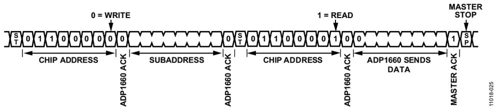
Figure 30. I<sup>2</sup>C Read Sequence for a Single Register
