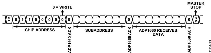
Figure 29. I<sup>2</sup>C Write Sequence for a Single Register
