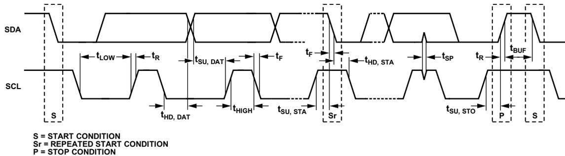
Figure 3. I<sup>2</sup>C-Compatible Interface Timing Diagram
