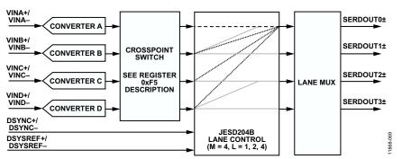
Figure 64. AD9656 Transmit Link Simplified Block Diagram
