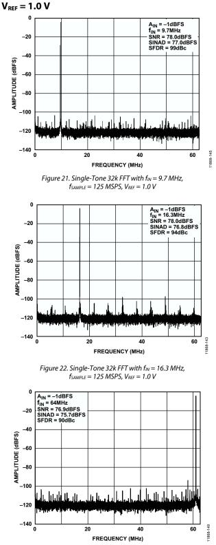
Figure 23. Single-Tone 32k FFT with  $f_{\rm IN}$  = 64 MHz,  $f_{\rm SAMPLE}$  = 125 MSPS,  $V_{\rm REF}$  = 1.0 V
