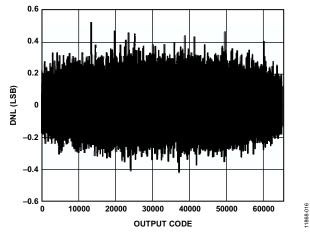
Figure 17. Differential Nonlinearity (DNL),  $f_{\text{IN}}$  = 9.7 MHz,  $f_{\text{SAMPLE}}$  = 125 MSPS,  $V_{\text{REF}}$  = 1.4 V
