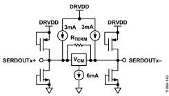
Figure 40. Equivalent SERDOUTx± Circuit
