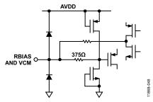
Figure 42. Equivalent RBIAS and VCM Circuit
