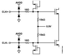
Figure 38. Equivalent Clock Input Circuit
