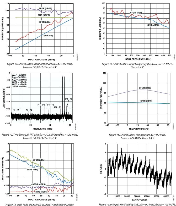
Figure 16. Integral Nonlinearity (INL), f<sub>IN</sub> = 9.7 MHz, f<sub>SAMPLE</sub> V<sub>REF</sub> = 1.4 V
