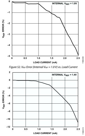
Figure 53.  $V_{REF}$  Error (Internal  $V_{REF} = 1.4$  V) vs. Load Current
