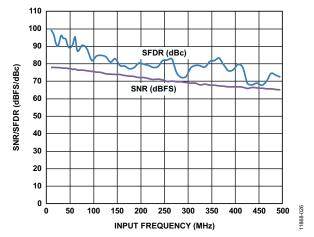
Figure 30. SNR/SFDR vs. Input Frequency (fin), f<sub>SAMPLE</sub> = 125 MSPS, V<sub>REF</sub> = 1.0 V
