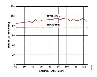
Figure 36. SNR/SFDR vs. Sample Rate,  $f_{IN} = 64 \text{ MHz}$ ,  $V_{REF} = 1.0 \text{ V}$
