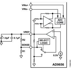
Figure 51. Programmable Internal Reference Configuration
