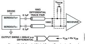
Figure 67. AC-Coupled Digital Output Termination Example
