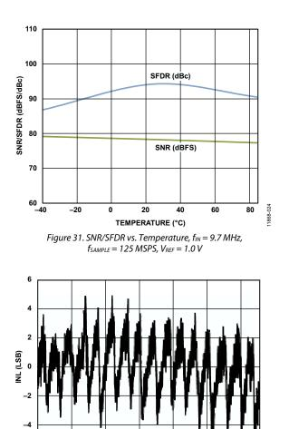
11868-009 0 10000 20000 30000 40000 50000 60000 OUTPUT CODE Figure 32. Integral Nonlinearity (INL),  $f_{IN} = 9.7 \text{ MHz}$ ,  $f_{SAMPLE} = 125 \text{ MSPS}$ ,
