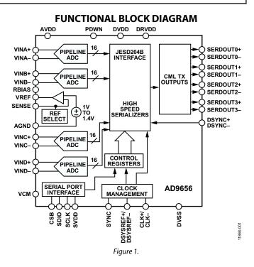
The AD9656 is available in an RoHS-compliant, nonmagnetic, 56-lead LFCSP.
