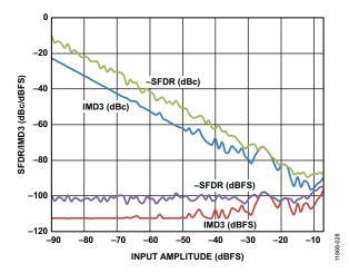
Figure 29. Two-Tone SFDR/IMD3 vs. Input Amplitude (A<sub>IN</sub>) with  $f_{IN1} = 70.5 \text{ MHz and } f_{IN2} = 72.5 \text{ MHz}, f_{SAMPLE} = 125 \text{ MSPS}, V_{REF} = 1.0 \text{ V}$
