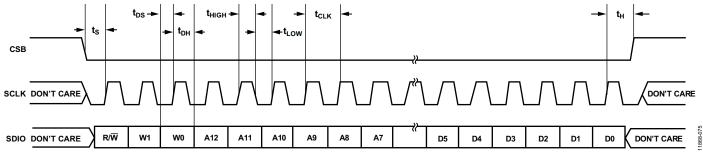
Figure 70. Serial Port Interface Timing Diagram
