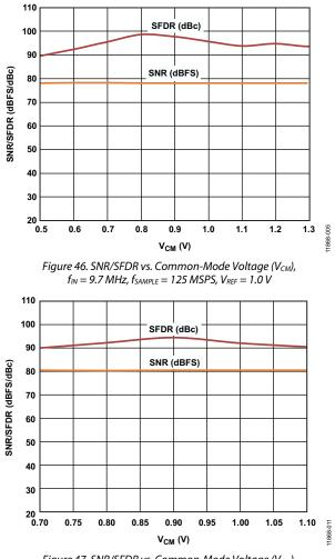
Figure 47. SNR/SFDR vs. Common-Mode Voltage ( $V_{CM}$ ),  $f_{IN} = 9.7 \text{ MHz}$ ,  $f_{SAMPLE} = 125 \text{ MSPS}$ ,  $V_{REF} = 1.4 \text{ V}$
