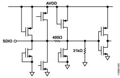
Figure 39. Equivalent SDIO Input Circuit
