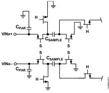
Figure 45. Switched-Capacitor Input Circuit
