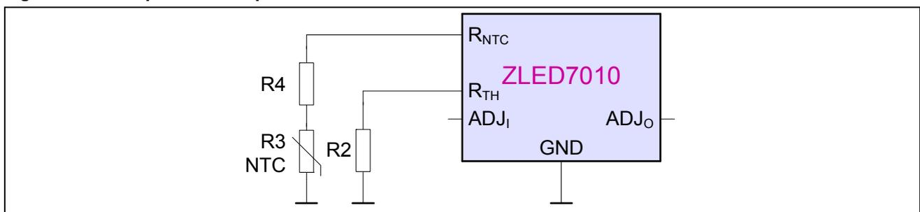
As shown in Figure 4.1, the temperature compensation curve is determined by R2, R3 (NTC) and R4. When the LED temperature increases, the resistance of R3 decreases. As R3 reaches the point that R3 plus R4 equal R2, the temperature compensation function starts to work by reducing  $I_{OUT}$ .
