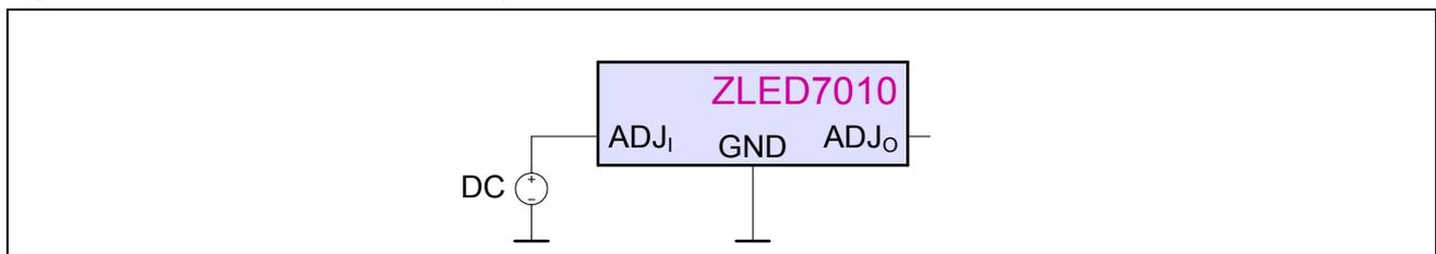
$$I_{OUT\_DC} = \frac{0.079 * V_{ADJ}}{R_S} \quad (2)$$
