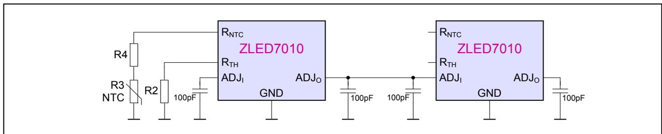
In Figure 5.2, note that each ZLED7010 can drive up to three slave ICs in the next stage. Using more than three stages to maintain current coherence is not recommended. Up to thirteen ZLED7010 can be connected in one system.
